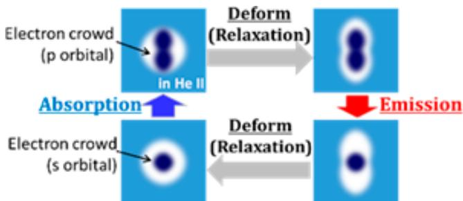
Fig. 1. Deformation cycle of an atomic bubble.
