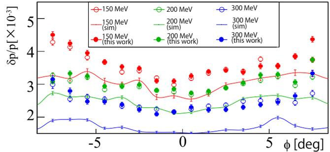
Fig. 2. Comparison of the momentum resolution between the measured map and the calculated one. The solid lines show the simulation results, the open circles show the results obtained with the calculation map, and the filled circles show the results obtained with the measured map. Red indicates the results with 150 MeV, green indicates the results with 200 MeV, and blue indicates the results with 300 MeV.
