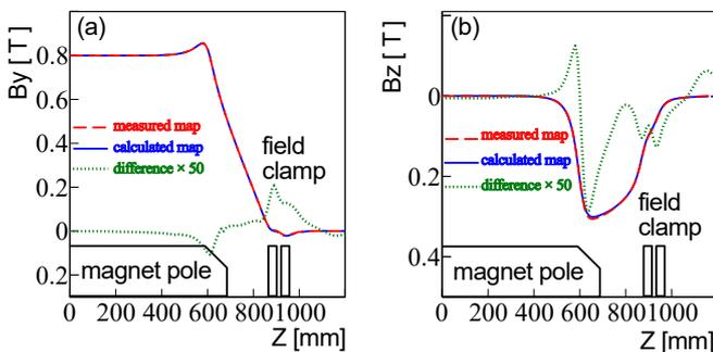
Fig. 1. Comparison between the measured map and the calculated one near the magnetic pole. The strength of the magnetic field was 0.8 T. (a) shows vertical component  $B_y$  and (b) shows horizontal component of the fringing field  $B_z$ . The red line is the measured map, blue line is the calculated one, and green line shows 50 times the difference between the two maps.
