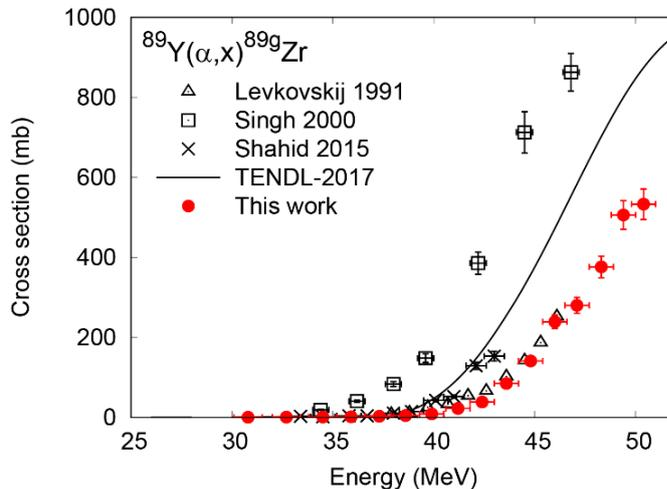
Fig. 1. Comparison of cumulative cross sections of the  $^{89}\text{Y}(\alpha, x)^{89g}\text{Zr}$  reaction with previously reported data<sup>3–5)</sup> and TENDL-2017 data.<sup>10)</sup>
