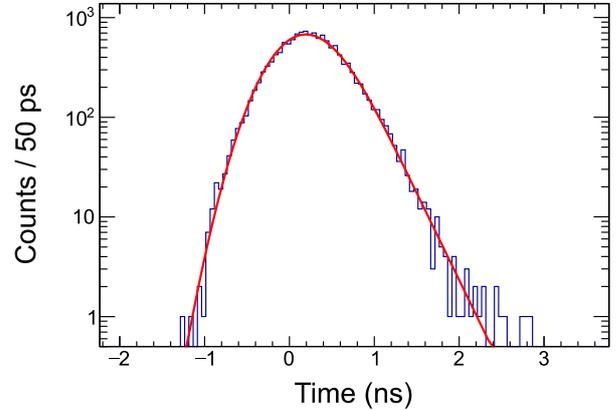
Fig. 2. Time spectrum of  $\gamma$ -ray signals following  $\alpha$ -particle signals for 4783.5-keV  $\alpha$  particles and 42.4-keV  $\gamma$  rays (histogram). A single exponential decay function convoluted with a Gaussian function is fitted to the data (curve).
