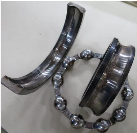
Fig. 1. Damaged bearing unit, disassembled from the coupling side of the motor unit.
