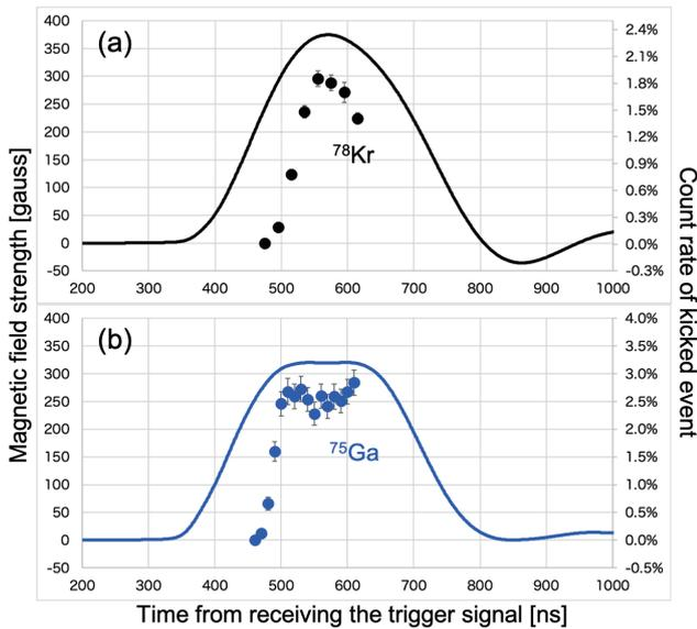
Fig. 1. Black line shows measured magnetic field, whereas blue line shows field experienced by particle (see text). Black and Blue dots indicate kicked events of <sup>78</sup>Kr and <sup>75</sup>Ga, respectively.
