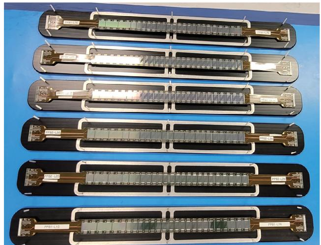
Fig. 2. Fully assembled INTT preproduction ladders.
