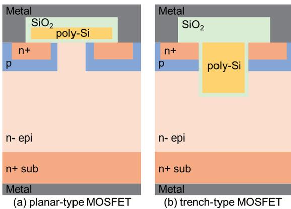
Fig. 1. Cross-sectional structure of the test devices.
