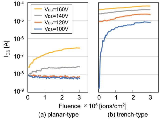
Fig. 2. Result of current monitoring during irradiation.
