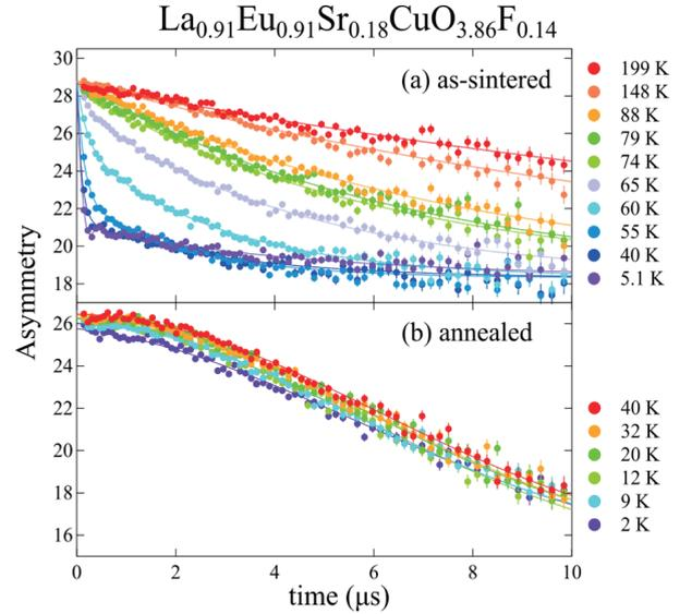
Fig. 1. Zero-field  $\mu\text{SR}$  time spectra of (a) as-sintered and (b) oxidation-annealed  $\text{La}_{1-x/2}\text{Eu}_{1-x/2}\text{Sr}_x\text{CuO}_{4-y}\text{F}_y$  with  $x = 0.18$  and  $y = 0.14$ .
