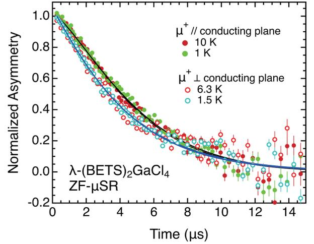
Fig. 1. Normalized ZF- $\mu$ SR time spectra with the setup of  $\mu^+$  injected parallel and perpendicular to the conducting plane. The solid lines represent fitting lines obtained using the stretched exponential function.
