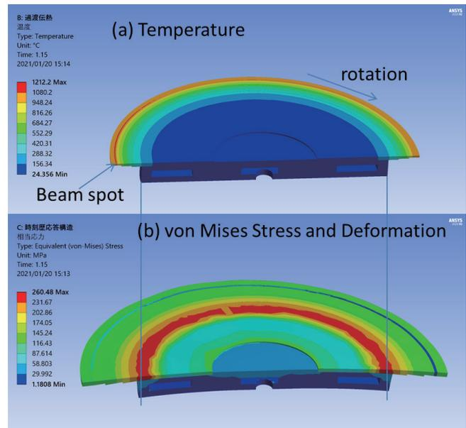
Fig. 1. Results of thermo-mechanical calculation of the rotating target. Only half of the simulation model is displayed in the figure to show the cross section of the target. (a) Temperature distribution of the target displayed in color on the original model shape (not deformed). (b) von Mises stress distribution displayed in color on the deformed shape. Deformation was magnified by a factor 50 so that the deformation can be viewed easily.
