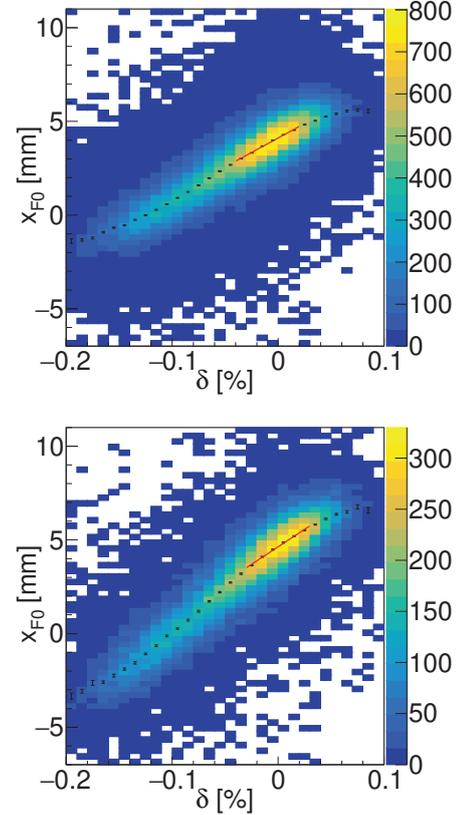
Fig. 1. Correlation between the deduced  $x$  and  $\delta$  at F0 for two different settings:  $(x|\delta)$ <sub>F0</sub> = 34.1 mm/% (upper panel) and  $(x|\delta)$ <sub>F0</sub> = 44.6 mm/% (lower panel). Fitting results obtained using linear functions are shown with red lines. Each slope corresponds to the deduced dispersion.
