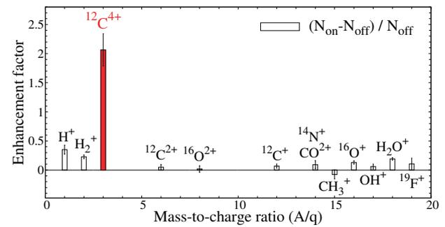
Fig. 3. Enhancement factors of extracted of  $^{12}\text{C}^{4+}$  ions.
