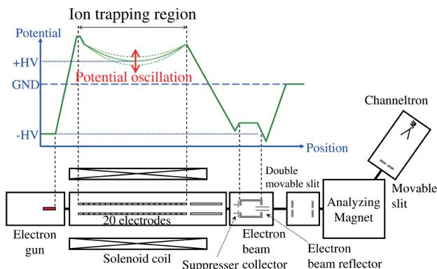
Fig. 1. The schematic diagram of the prototype RECB.
