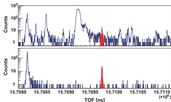
Fig. 2. Measured TOF spectrum without and with the cleaning mode; spectral peak marked in red is <sup>82</sup>Ge.
