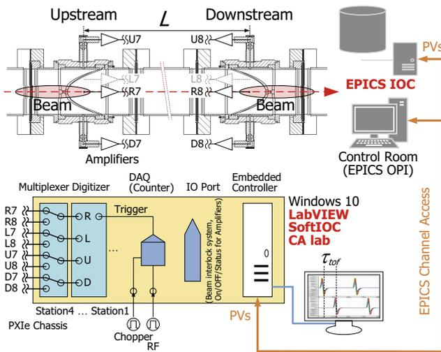
Fig. 1. Block diagram of the BEPMs and DAQ.
