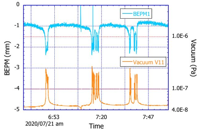
Fig. 2. Measured results showing the relationship between the beam position at BEPM 1 and the vacuum between cryomodules of CM1 and CM2.
