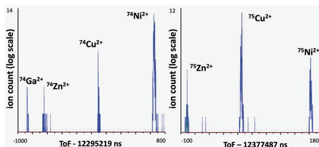
Fig. 2. New ion time-of-flight spectra of the  $A = 74$  isobars Ga, Zn, Cu, and Ni in the left part, and  $A = 75$  isobars Zn, Cu, and Ni produced from on-line beam centered on  $^{79}\text{Ni}$  and also from in-trap decay.
