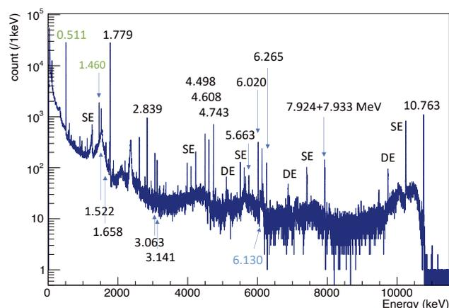
Fig. 2.  $\gamma$ -ray energy spectrum measured by GX5019 suppressed by a Compton suppressor. The  $\gamma$  rays from 511 keV to 10.7 MeV can be observed. In the spectrum, SE (DE) means single (double) escape peaks corresponding  $\gamma$ -rays.
