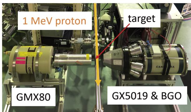
Fig. 1. Photograph of the experimental setup. Two Ge detectors were set next to the target and at an angle of 90-degrees to the beam.
