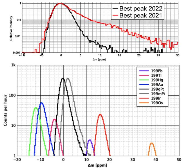
Fig. 1. (top) Comparison of MRTOF peak shape from 2021 with the improved peak shape achieved in 2022. (bottom) Simulated spectrum for  $A = 199$  isobars based on measured MRTOF peak shape and calculated production yields. Prior to improving the peak shape it was very difficult to observe  $^{199}\text{Ir}$  ions as they produced only a small fluctuation in the tail of the  $^{199}\text{Pt}$  ion peak.
