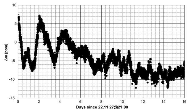
Fig. 2. Drift of the peak position over 16 days of measurement while roughly regulating the MRTOF chamber at  $38^\circ\text{C}$ . The maximum fluctuation is consistent with a thermal fluctuation of  $\Delta T_{pk-pk} \approx 0.75$  K.
