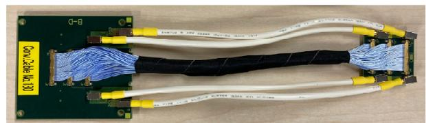
Fig. 3. Readout cables for the INTT ladder based on the  $\mu$ -coax technology.
