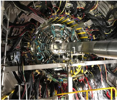
Fig. 1. Installed TPC in the sPHENIX detector.
