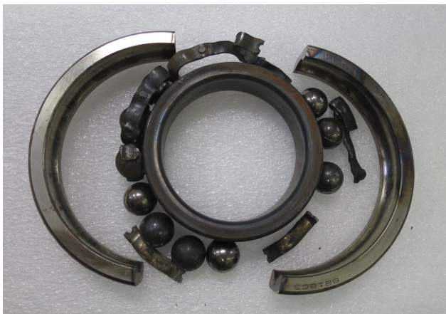
Fig. 1. Damaged bearing unit, disassembled from the coupling side of the motor unit.
