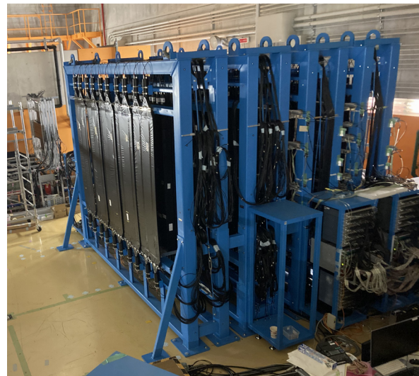
Fig. 2. View of the NEBULA-Plus array, including the veto detectors, prior to the installation of the electronics.
