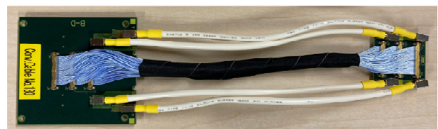
Fig. 3. Readout cables for the INTT ladder based on the \mu -coax technology.
