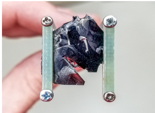
Fig. 1. An image of the sample of single-crystal CuO used in the present experiment.
