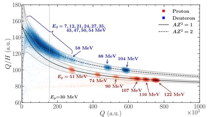
Fig. 2. Correlation between  $Q/H$  and  $Q$ . Proton (red) and deuteron (blue) loci are clearly separated. Lines show the calibrated response function depending on  $AZ^2$ . The hatched area represents the interpolated  $2\sigma$  region.
