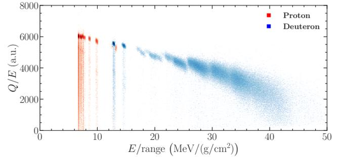
Fig. 1.  $Q/E_{p(d)} (\propto dL/dE)$  plot as a function of  $E_{p(d)}/\text{range} (\sim \langle dE/dx \rangle)$ . Red and blue points correspond to protons and deuterons data, respectively. The spots are correspond to the data acquired in each magnetic field settings of GR.
