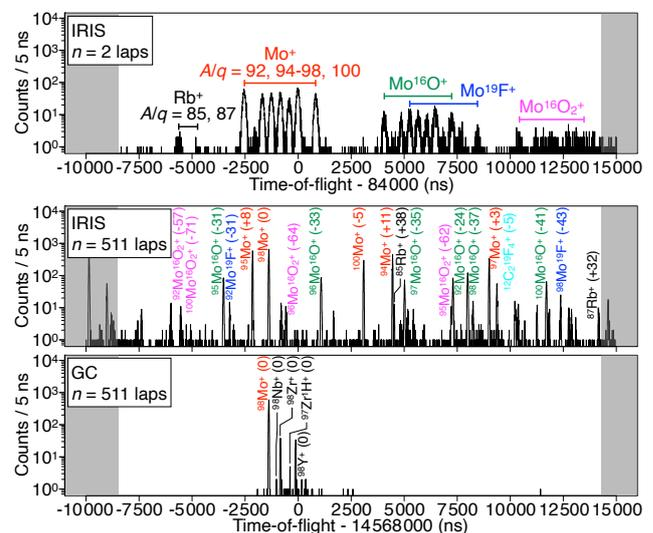
Fig. 2. TOF spectra obtained with MRTOF-MS. Top: At 2 laps from the IRIS side. Middle and Bottom: At 511 laps for  $^{98}\text{Mo}^+$  from the IRIS side and the GC side with only  $A/q = 98$  ions selected by an in-MRTOF deflector, with peak assignments for major peaks. The lap differences for those peaks from 511 laps are described in brackets. The gray regions are disturbed by high-voltage switching.
