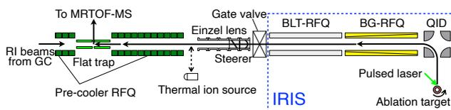
Fig. 1. Schematic of IRIS and the ion trap system on MRTOF-MS.
