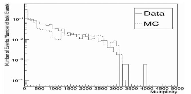
Fig. 1. Comparison of the cluster multiplicity distributions of the INTT inner barrel (solid line) and result of the MC simulations (dashed line).
