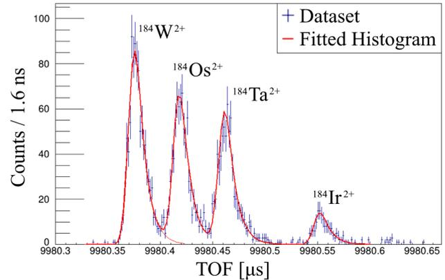
Fig. 1. TOF histogram of  $A = 184$  isobars measured in MRTOF after drift correction. Four peaks are fitted (red) using the hyper-EMG function.
