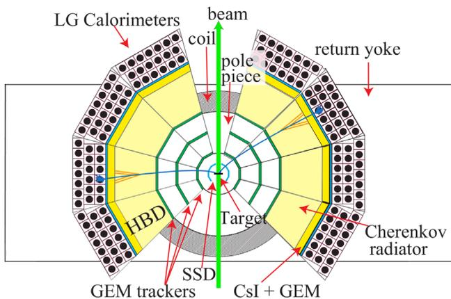
Fig. 1. Cross-sectional plan view of the E16 spectrometer in the eight-module configuration for Run-1, and operated in June 2023 for the first time.
