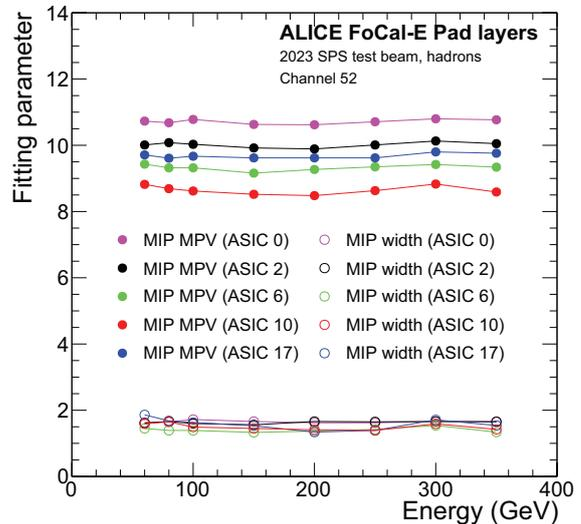
Fig. 2. Estimated MPVs and widths of the MIP distribution depending on the beam energy and pad layer.
