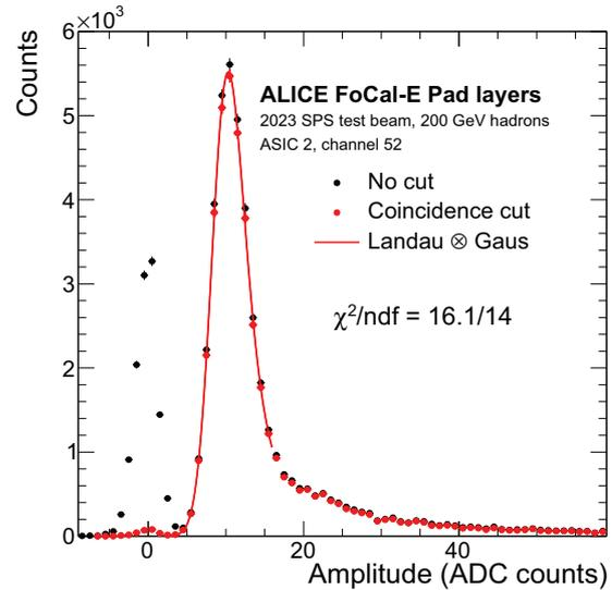
Fig. 1. MIP distribution for 200 GeV hadrons before (black) and after (red) the coincidence cut.
