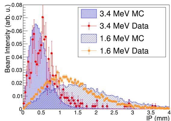
Fig. 2. A comparison of IP distributions between the data and MC simulations for 1.6 and 3.4 MeV  $\text{H}^+$  beams at an irradiation distance of 10 mm.
