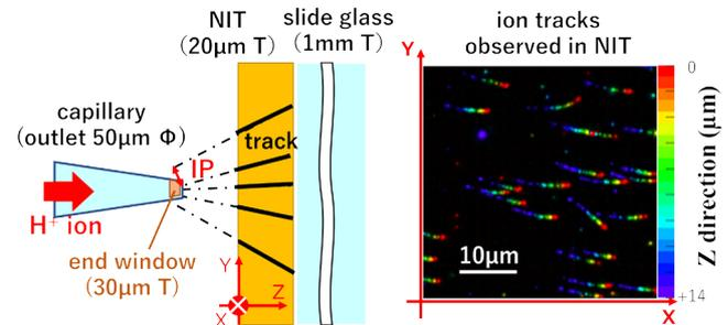
Fig. 1. A schematic of MeV ion beam irradiations to the NIT with the glass capillary. The right photograph shows an actual optical microscope image of ion tracks. The Z coordinate is displayed with a colored scale.
