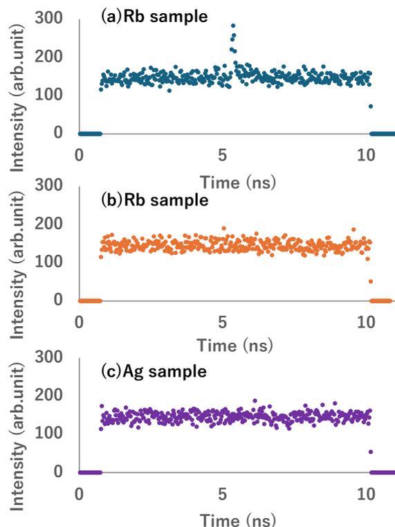
Fig. 2. TCSPC signals for Rb sample (a) with and (b) without ablation, and (c) for Ag sample ablation. Monochromator wavelength for three data points is 785 nm, which is shorter than the emission center wavelength of 793 nm.
