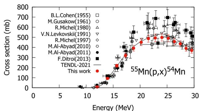
Fig. 1. Cross sections of the <sup>55</sup>Mn( $p, x$ )<sup>54</sup>Mn reaction compared with the previous studies found in the EXFOR library<sup>5)</sup> and the TENDL-2021 values.<sup>6)</sup>
