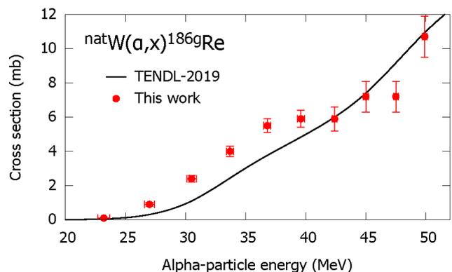
Fig. 1. Cross sections of the  $^{nat}\text{W}(\alpha, x)^{186g}\text{Re}$  reaction with the TENDL-2019 value.
