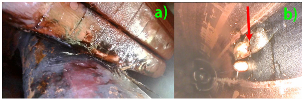
Fig. 1. Outside view of the downstream side of MDC3 (a) and the inside of the beam duct (b). Melting point is indicated by the red arrow.
