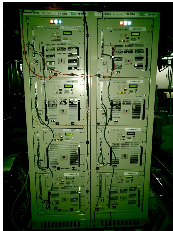
Fig. 1. Photograph of two power supply enclosures installed in the RILAC accelerator room, with four power supplies installed per enclosure.
