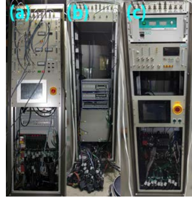
Fig. 1. Rf control system for the RRC resonator no.1 before (a), during (b), and after modification (c). Same for no.2 system.
