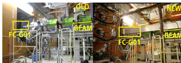
Fig. 1. External view of the old Faraday cup at the exit of the SRC (left panel) and new high-intensity Faraday cup (right panel).
