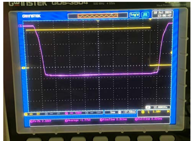
Fig. 2. Oscilloscope trace showing the rising and falling transition of the slow photodiode switch used to gently turn the detector bias on and off. Yellow trace is the switch trigger signal, purple trace is the switch output signal. Time scale is 5 ms per division.
