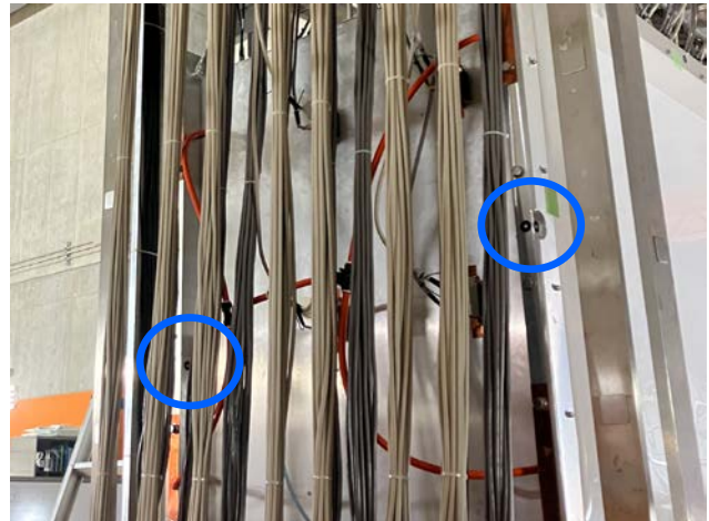
Fig. 1. Photograph of the FDC2. Markers in bad positions are circled. Left one is located behind cables. Two on the right are too close to distinguish. The markers attached to the scribed lines are still recommended.
