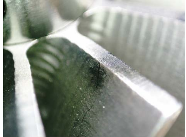
Fig. 1. T2 compressor wheel with scratches.
