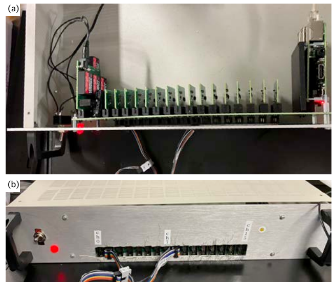
Fig. 1. Second prototype device with 16 channels. (a) top view (b) front panel view.
