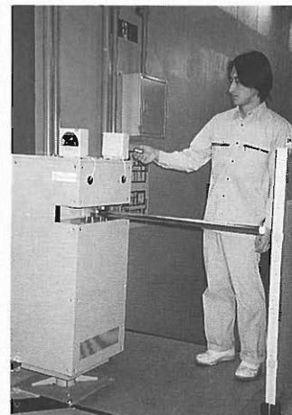
Fig. 2. Photograph of new FB-readers on top of the gate-bar at the entrance of experimental vault.
