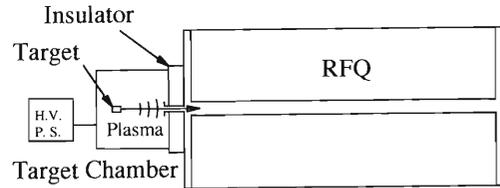
Fig. 1. Schematic view of the direct injection method.
