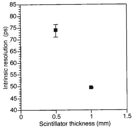
Fig. 2. Intrinsic time resolution of PMT coupled to large scintillator by a light guide.
