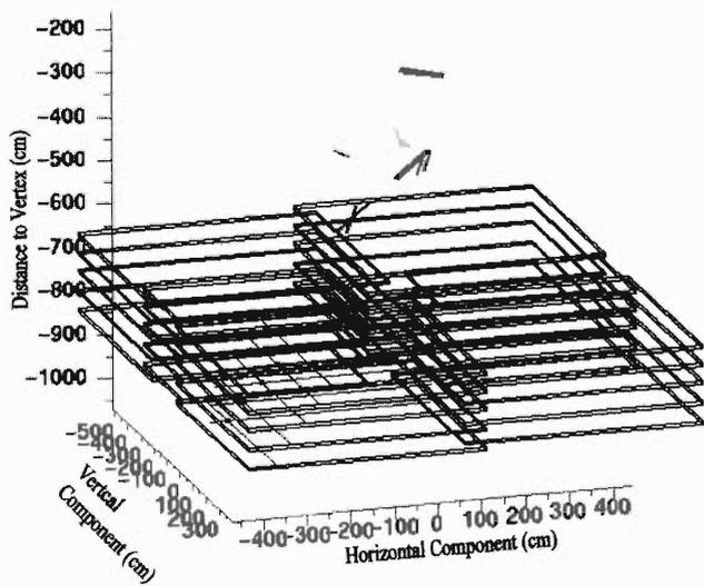
Fig. 3. Cosmic ray track in the South Muon Arm.
