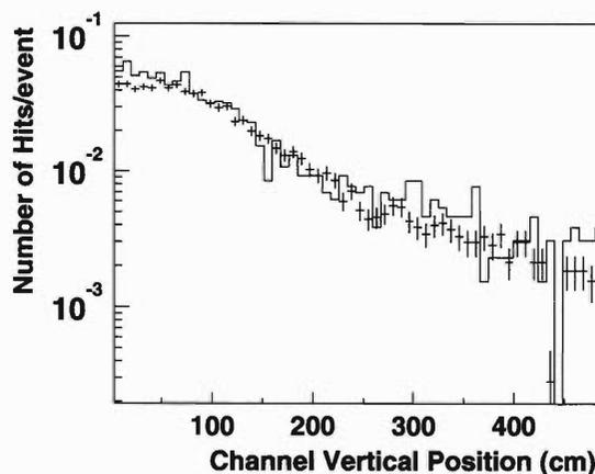
Fig. 2. Number of hits per event for each channel on the 4th horizontal plane, upper West panel. Lines indicate simulation and points indicate real data with statistical errors.
