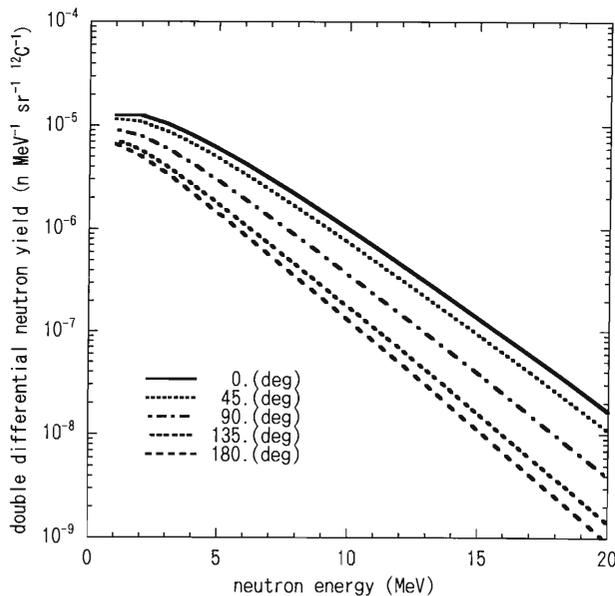
Fig. 1. Neutron spectra of 6.25-MeV/nucleon  $^{12}\text{C}$  beam bombardment on a full-stop copper target.
