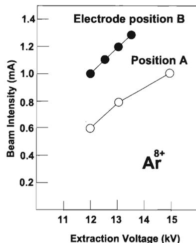
Fig. 2. Beam intensity of Ar<sup>8+</sup> as a function of extraction voltage at electrode positions A and B.
