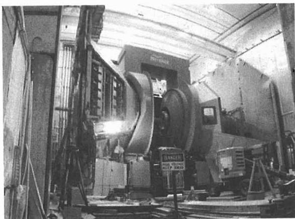
Fig. 1. Three stations of cathode strip chambers and their front-end electronics for the south muon tracker have been installed in the south muon magnet (left in the picture). The north muon tracker (right) will be installed in the summer of 2001.
