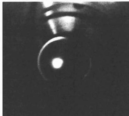
Fig. 1. A typical beam profile of the  $N^{4+}$  ion beam at 100 eV/q obtained by the CCD camera.
