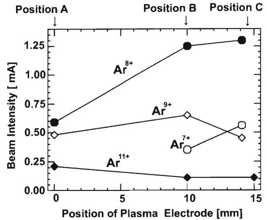
Fig. 3. Beam intensity of various charge states of Ar ions as a function of plasma electrode position.
