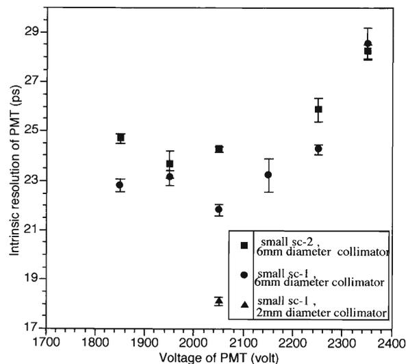
Fig. 1. Intrinsic time resolution of PMT directly coupled to small scintillator.
