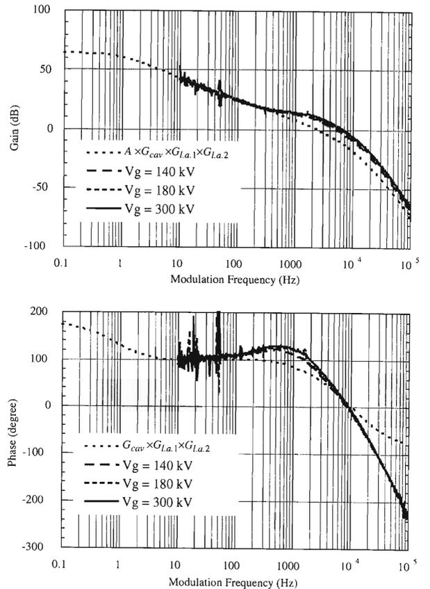
Fig. 4. Bode diagrams of the open-loop transfer functions of the rf-amplitude modulation. Solid and dashed curves are the measured ones. The dotted curve is the calculated transfer function, which is given by the cavity and the two loop amplifiers in Fig. 1. In the calculation, the loaded Q-value of the cavity response was set for the measured value of 12,500.
