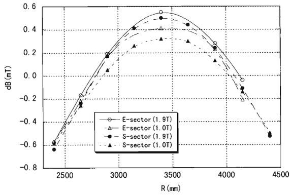
Fig. 4. Change of the magnetic fields along the sector centerline when the beam chamber was evacuated.
