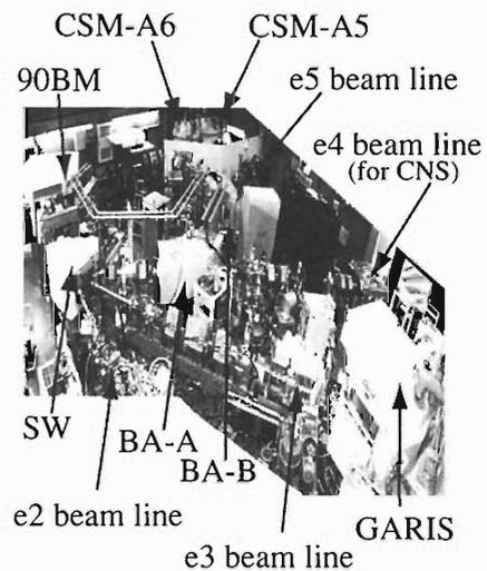
Fig. 2. Photograph of the CSM A5–A6 cavities, the beam lines e1–e5 and the GARIS in the No. 1 target room.
