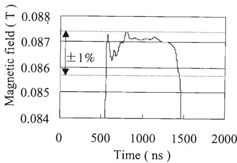
Fig. 4. Magnetic field at the flat-top with the capacitors.
