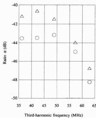
Fig. 4. Ratio of the amplitude at the dee voltage pickup to that at the feeder of the flat-top resonator. Circles represent the ratio of the No. 1 resonator and triangles represent that of the No. 2 resonator.
