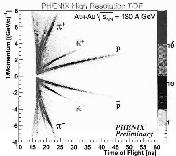
Fig. 1. Contour plot of the time-of-flight versus inverse momentum.
