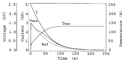
Fig. 2. Current,  $I$ , maximum temperature,  $T_{max}$ , the maximum voltage difference inside the coil,  $V_{max}$  and voltage drop across the dump resistor,  $R_m I$  of the superconducting main coil of SRC during quench, in the case of  $R_m = 0.3 \Omega$  (Run#1 in Table 1).
