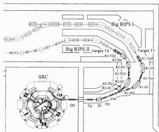
Fig. 2. Schematic layout of the beam transport line from SRC to Big RIPS separators.
