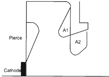
Fig. 2. Cross-sectional view of previous anode shape (A1) and modified anode shape (A2).
