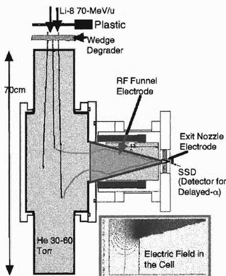
Fig. 1. Diagram of the rf ion guide on-line test setup.
