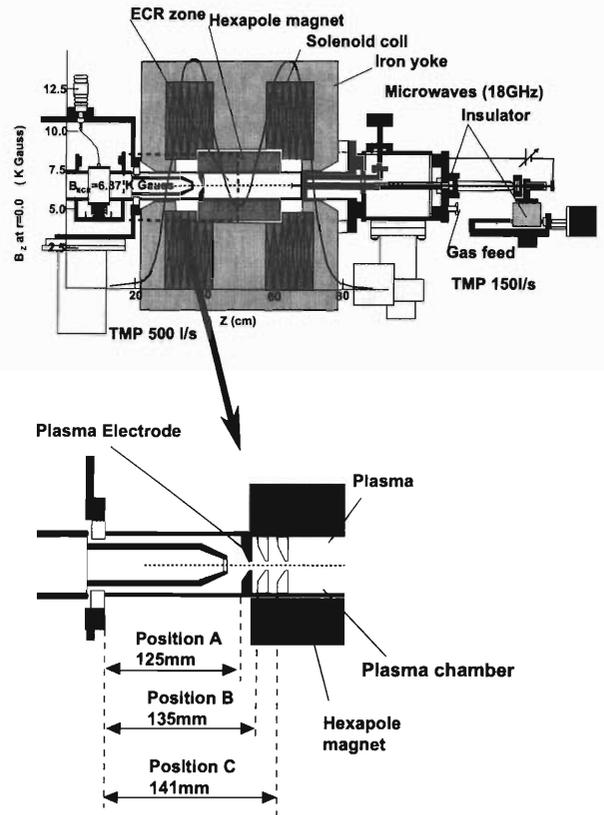
Fig. 1. Cross-sectional view of RIKEN 18 GHz ECRIS and its plasma chamber.
