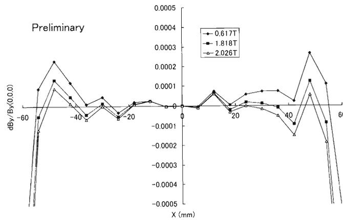
Fig. 4. Uniformity of the magnetic field.
