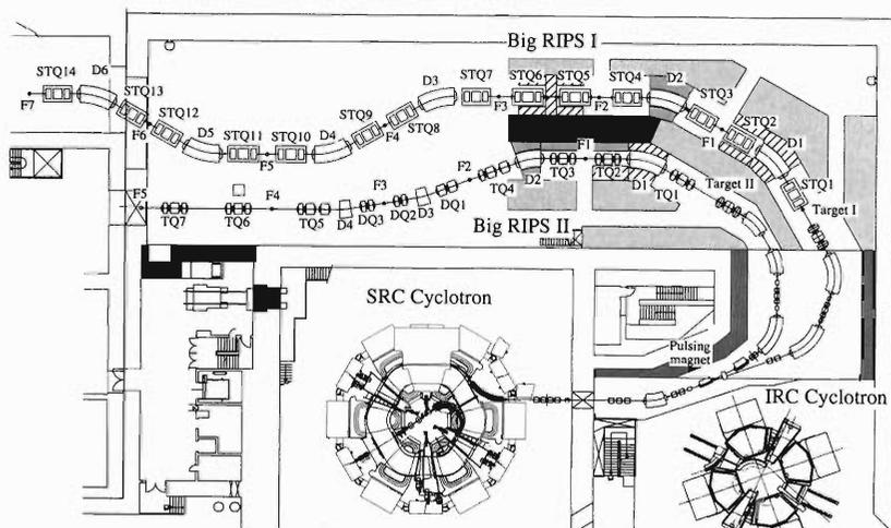
Fig. 1. A schematic layout of the BigRIPS separator. Quadrupole magnets are indicated by STQ<sub>n</sub>, TQ<sub>n</sub> and DQ<sub>n</sub>, while dipole magnets are indicated by D<sub>n</sub>. F<sub>n</sub> denotes focuses.
