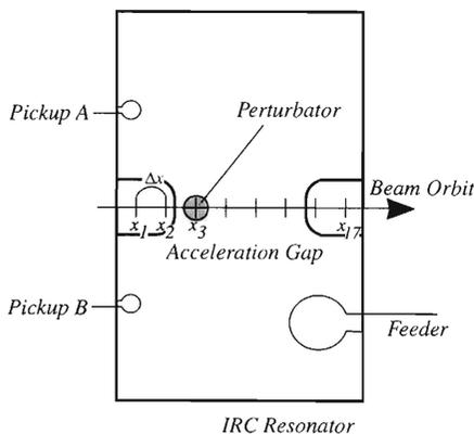
Fig. 2. Setup of the phase-shift measurement.
