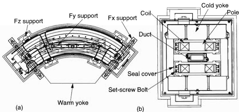
Fig. 1. (a) Plan view and (b) cross-sectional view of the SBM.
