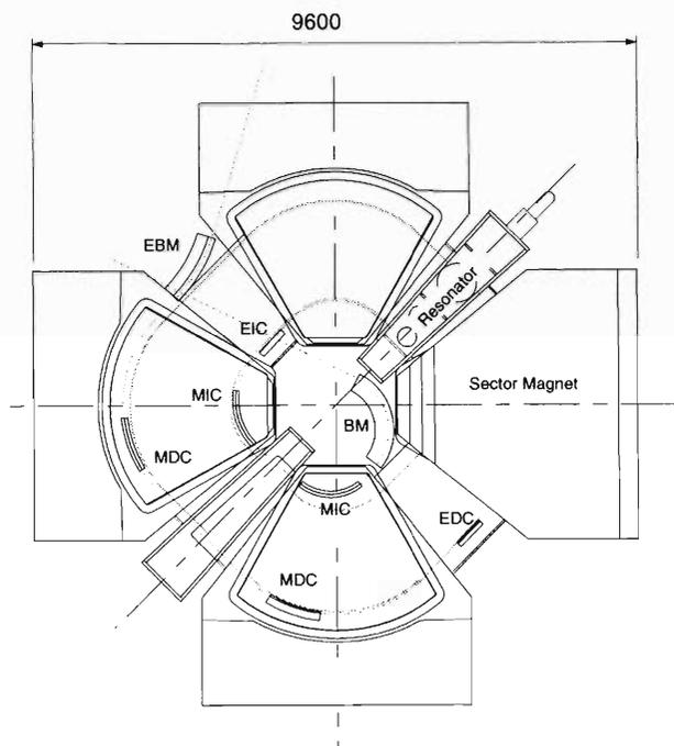
Fig. 3. Conceptual plan view of the fRC.
