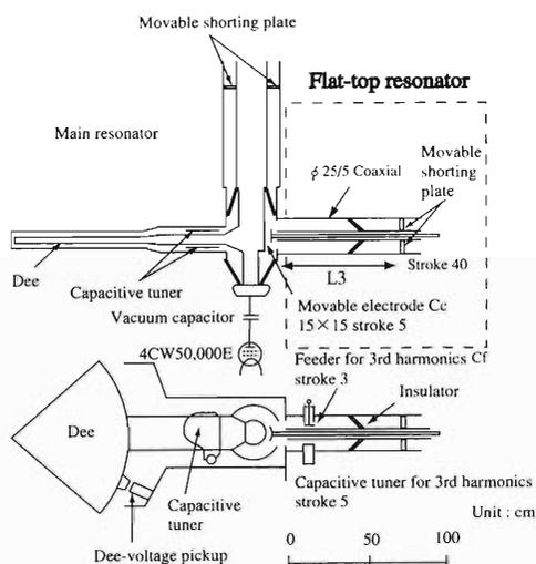
Fig. 1. Cross-sectional view of the flat-top acceleration system for the RIKEN AVF Cyclotron.
