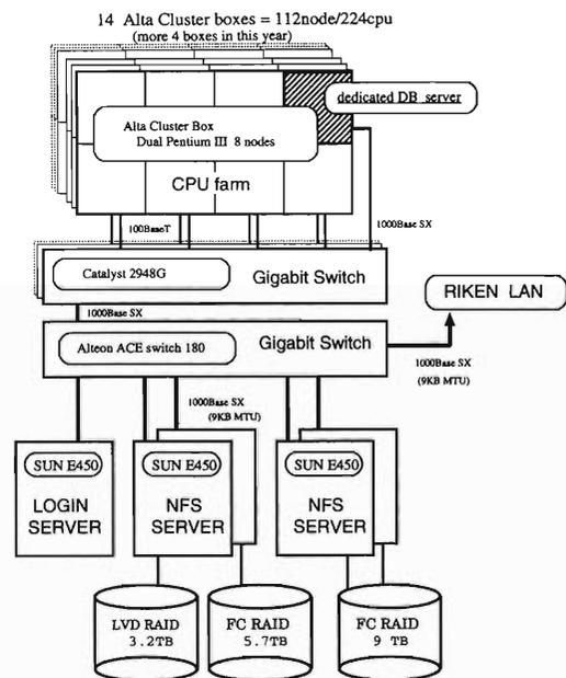
Fig. 1. Current CCJ system configurations.
