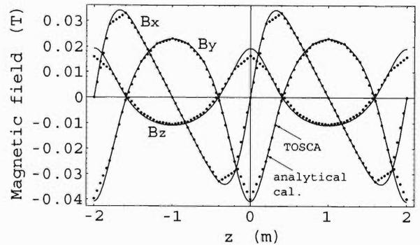
Fig. 4.  $B_x(z)$ ,  $B_y(z)$ , and  $B_z(z)$  due to iron, along a line of  $x = 0.15$  m and  $y = 0$ .
