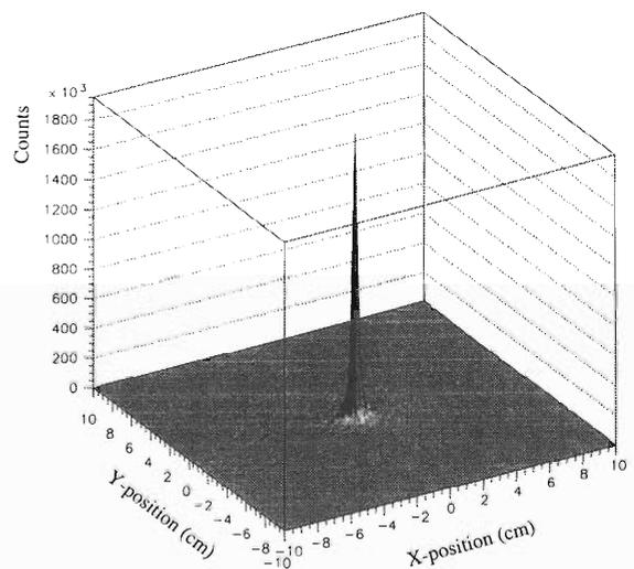
Fig. 2. X-Y plot for the center point source. A  $200 \times 200 \text{ mm}^2$  image plane with 2 mm pixels was used for the reconstructions, with 1000 Compton scatter events. The resolution (FWHM) is 4 mm in the X- and Y-directions.
