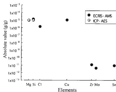
Fig. 2. Relative abundances of trace elements for  $\text{Al}_2\text{O}_3$  rod of 99.99% purity are compared in results of ECRIS-AMS with ICP-AES.
