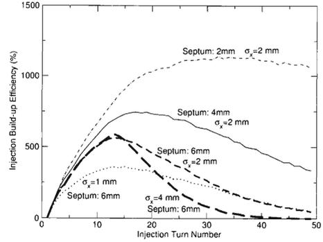
Fig. 4. Multiturn injection efficiency of the ACR for several septum thicknesses (2 mm, 4 mm, 6 mm) and horizontal sizes of the injection beam ( $\sigma_x = 1$  mm, 2 mm, 4 mm).
