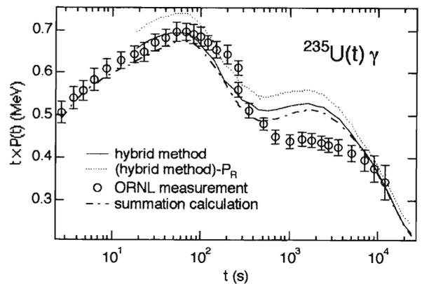
Fig. 1. Decay heat power from a pulse thermal fission of  $^{235}\text{U}$ . The solid (dotted) line shows the decay heat power calculated using the hybrid method with (without) a correction term. Also shown for comparison are the results of ORNL measurements (open circles with error bars) and summation calculations with ENDF/B-VI (dash-dotted line).
