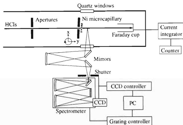
Fig. 1. Schematic drawing of the experimental setup installed in the hall for slow highly charged ions at RIKEN.
