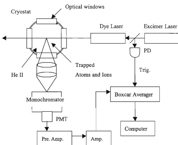
Fig. 1. Schematic of optical detection.
