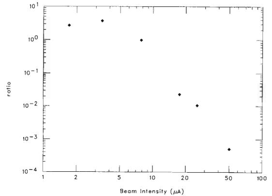
Fig. 5. The current of  ${}^4\text{He}^{2+}$  ions which passed through the liquid film divided by the current of  ${}^4\text{He}^+$  ions which passed by the liquid film as a function of beam intensity measured by a Faraday cup placed upstream of the stripper. The disc was rotated at 1500 rpm.
