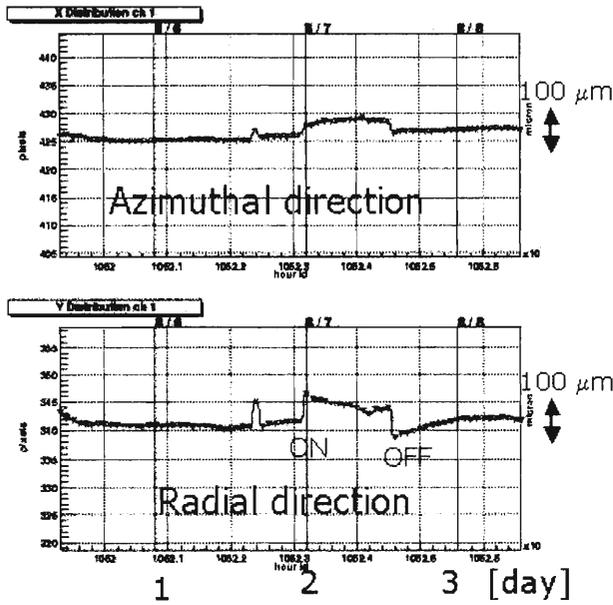
Fig. 2. History of focal image position for azimuthal direction (upper) and radial direction (lower). In the middle of the measured period in the plot, a  $60\ \mu\text{m}$  position shift caused by the spectrometer magnet ON/OFF was detected.
