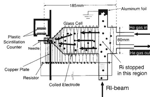
Fig. 1. Schematic view of the setup. (The copper plates are the shield for  $\beta$ )
