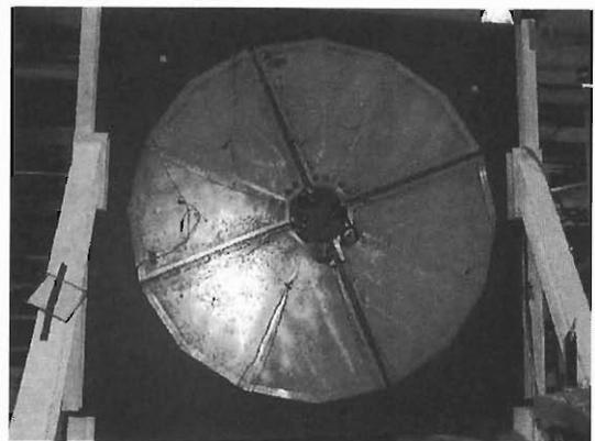
Fig. 2. Station 1 is built in four quadrants but is electrically divided into octants to match the octants of stations 2 and 3.
