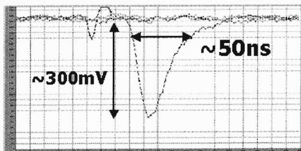
Fig. 1. A typical waveform from CNI recoil carbons.
