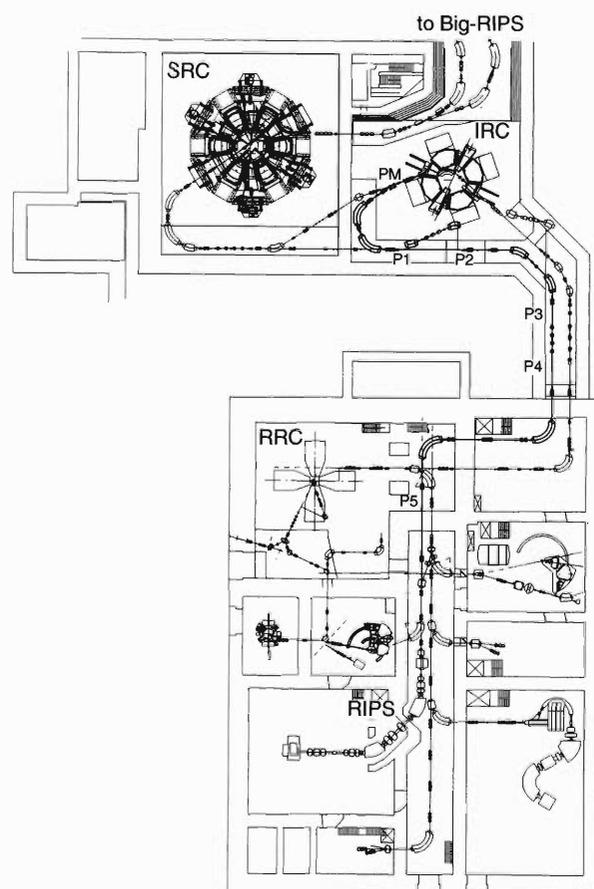
Fig. 1. The beam line from IRC to RARF is shown in bold. The PM indicates the pulsing magnet introduced for the time-sharing of beams.
