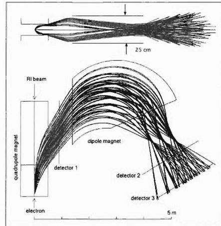
Fig. 1. Proposed electron spectrometer for the eRI collider of MUSES.
