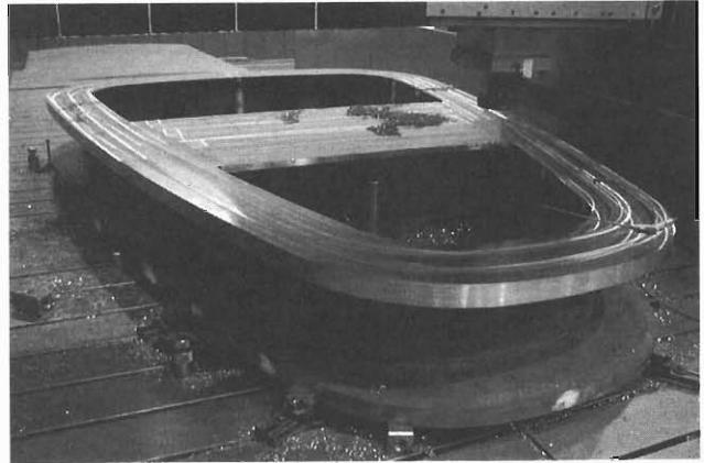
Fig. 2. Photograph of machining a main coil vessel.
