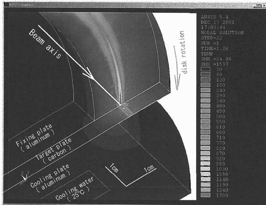
Fig. 2. Cross-sectional view of the temperature distribution in the target disk near the  $^{238}\text{U}$  beam spot.
