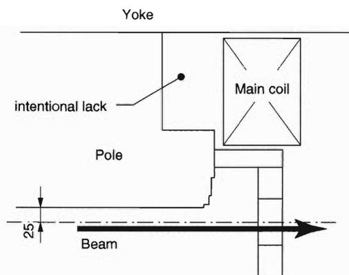
Fig. 2. Schematic cross-sectional view of the pole.
