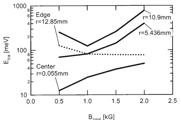
Fig. 1. Transverse electron temperature in the cooling section calculated by SAM (dotted lines) and EGUN (solid lines). The value of  $r$  indicates the radial beam position at the dispenser cathode.
