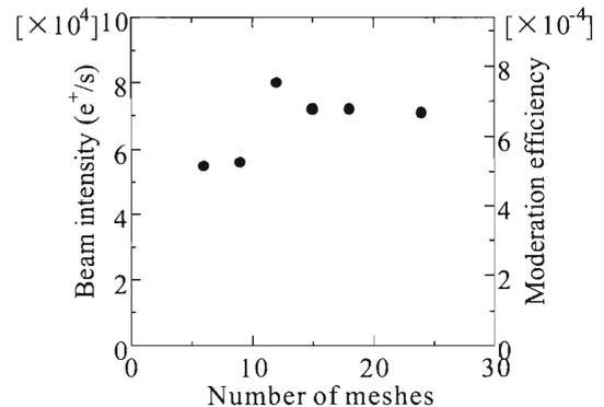
Fig. 1. Slow positron beam intensity plotted versus number of overlapping tungsten meshes of the moderators. The activity of the  $^{22}\text{Na}$  source is  $1.38 \times 10^8 \text{Bq}$  (3.73mCi). The scale on the right side indicates the moderation efficiency.
