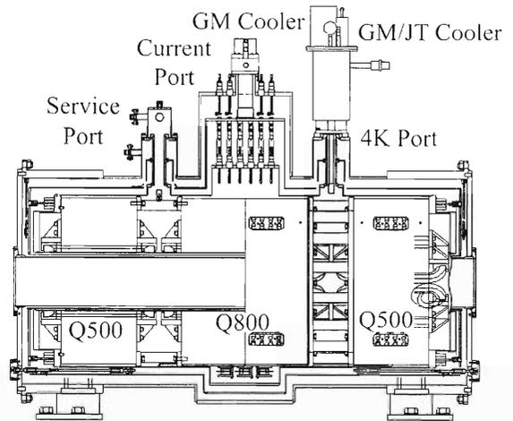
Fig. 1. Quadrupole triplet with small refrigerators.
