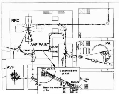
Fig. 1. Layout of AVF-PA beam line. A vertical view of the skew beam line is shown in the rectangular box.
