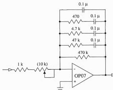
Fig. 2. Schematic drawing of a loop amplifier in the CSM level controller,<sup>2)</sup> denoted by Loop Amplifier-1 in Fig. 1.
