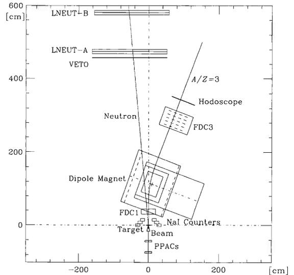
Fig. 1. Experimental setup of breakup experiments on  $^{11}\text{Li}$ ,  $^{14}\text{Be}$  and  $^{17}\text{B}$ .
