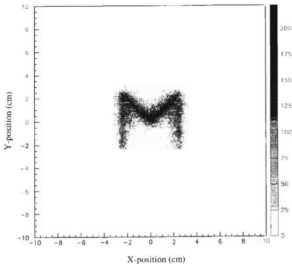
Fig. 3.  $X$ - $Y$  plot for a uniformly distributed volume source in the form of the letter M. The size of the M is  $50 \times 50 \text{ mm}^2$ . Six thousand events were used for the image.
