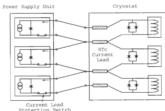
Fig. 2. Excitation circuit of the quadrupole triplet.
