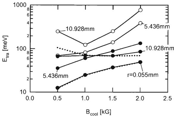
Fig. 3. Dependence of the transverse temperature on the magnetic field in the cooling section. Open and solid circles indicate the cases of A1 and A2, respectively. Dotted lines for  $E_{tra}$  show the results calculated by SAM in the case of A2.
