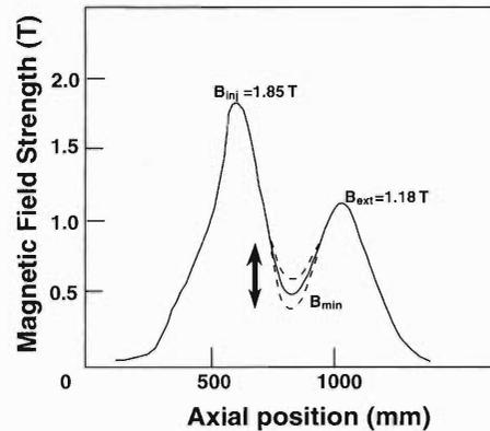
Fig. 3. Typical magnetic configuration for producing the Kr ions.
