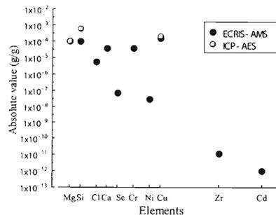
Fig. 1. Relative abundances of trace elements for  $\text{Al}_2\text{O}_3$  rod of 99.5% purity are compared in results of ECRIS-AMS with ICP-AES.
