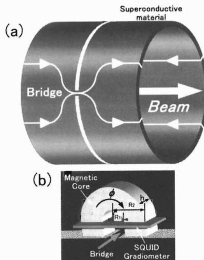
Fig. 1. (a) Schematic drawing of the superconductive CCC that we are designing. (b) Structure of the SQUID gradiometer and the magnetic core near the bridge.
