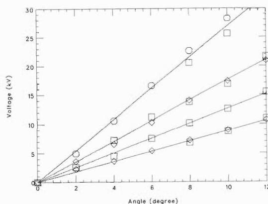
Fig. 3. Sorted helium ions by electrostatic deflector according to their energy and charge states. The horizontal axis indicates the deflection angle, and the vertical axis indicates the voltage of the deflector. Squares and diamonds indicate the data measured with a liquid film produced by 1600 rpm disc rotation and a  $80 \mu\text{g}/\text{cm}^2$  carbon foil,<sup>a</sup> respectively. Circles indicate the data obtained without any stripper.
