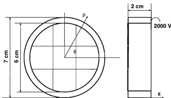
Fig. 1. Illustration of a segmented Ge detector manufactured by Eurisys Mesures. Its coordinate system is also presented.
