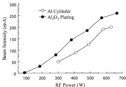
Fig. 1. Beam intensity of  $\text{Ar}^{11+}$  as a function of RF power. Open and closed circles are the results by using Al cylinder method and  $\text{Al}_2\text{O}_3$  plating method, respectively.
