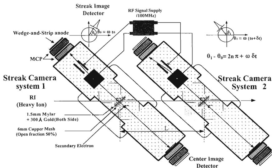
Fig. 1. Schematic of the ToF detector system.
