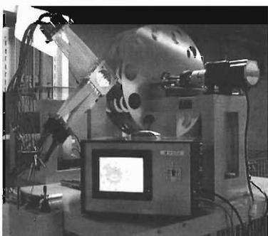
Fig. 1. Target wheel apparatus and detector array (exposed for clarity).
