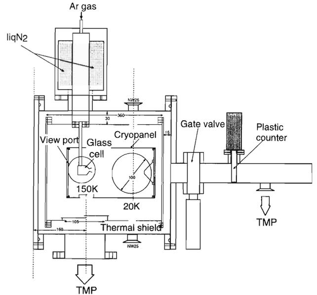
Fig. 1. Schematic view of the setup. The  $^{17}\text{N}$  beam is incident at the cell from the direction perpendicular to the figure, and a fraction of atoms in the beam are stopped in a gas in the cell. **TMP**: Turbomolecular pump.
