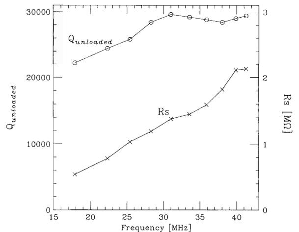
Fig. 4.  $R_s$  and unloaded Q-values as a function of frequency.
