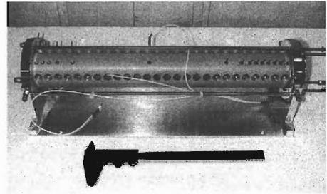
Fig. 1. Main body of the MR-TOF. Inside a plastic tube there are 15 gold-coated aluminum ring-electrodes as ion mirrors and lenses.
