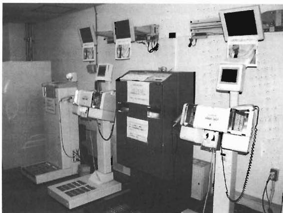
Fig. 1. The hand-foot-clothes monitors installed in the contamination test room of the Nishina Building.
