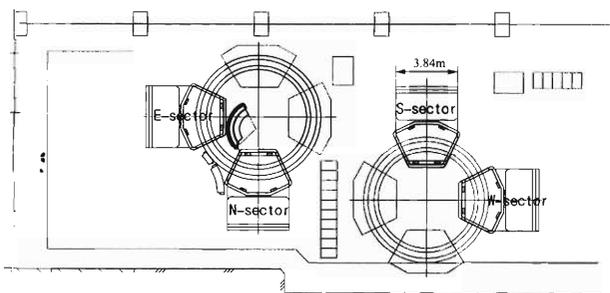
Fig. 1. Arrangement of the IRC sector magnets when the magnetic field measurements were carried out at Niihama factory.
