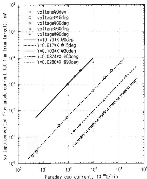
Fig. 1. Anode current response to the He beam current. The monitor was placed 1 m from the target, and the anode current was converted to voltage.
