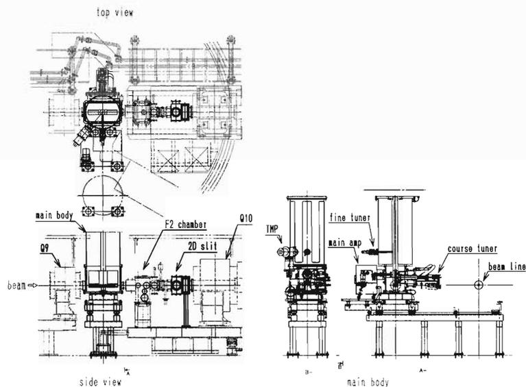
Fig. 1. The general plan for RF deflector system.
