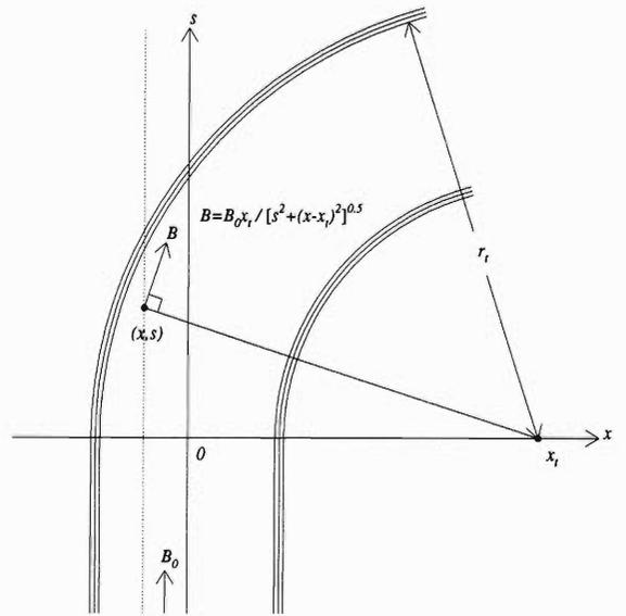
Fig. 3. Toroid structure idealized for calculation of the field.
