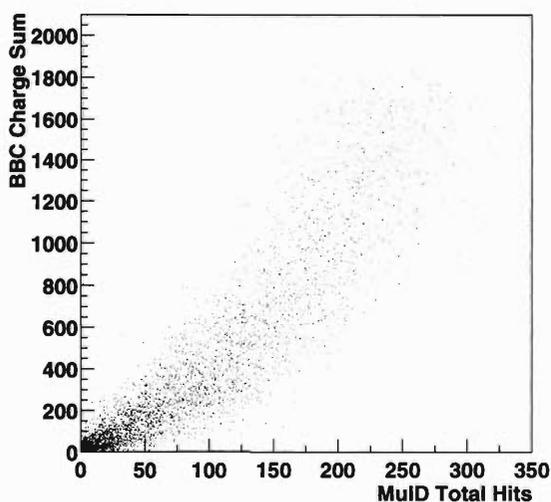
Fig. 1. Correlation between the total number of hits in MuID and the charge sum in the beam-beam counter (BBC).
