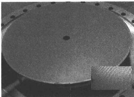
Fig. 4. New rf electrode assembly made of planar PCB. Part of the electrode is enlarged at the bottom right. An additional small central electrode will be attached at the center.
