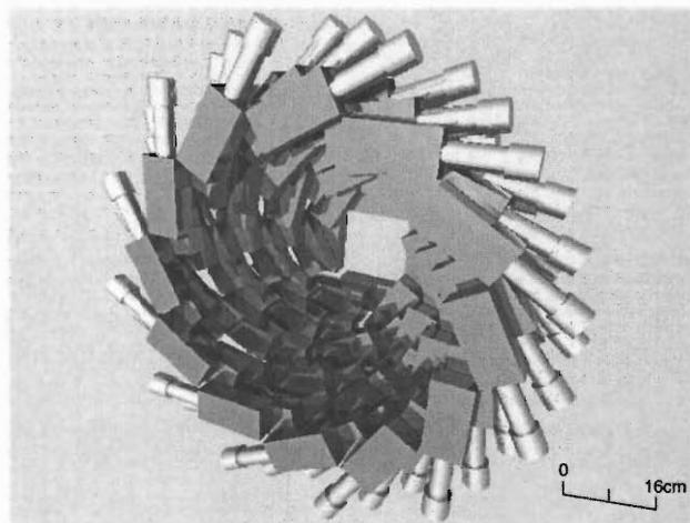
Fig. 1. Schematic of half of the NaI(Tl) array which consists of 80 crystals.
