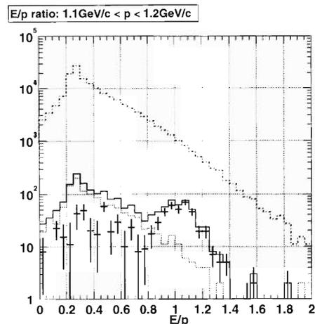
Fig. 2. Ratio of energy and momentum for all Drift Chamber (DC) tracks.
