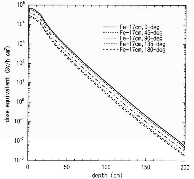
Fig. 2. Dose equivalent distribution in a 17-cm-thick-iron+183-cm-thick-ordinary-concrete slab. The irradiating neutrons are produced by 6.25-MeV/nucleon  $^{12}\text{C}$  beam bombardment on copper.
