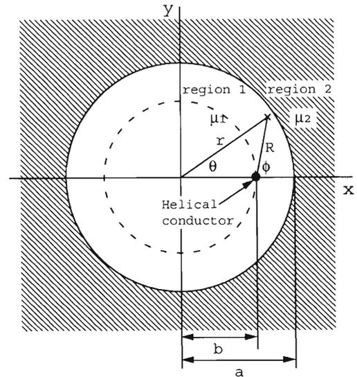
Fig. 2. Cross section of a single helical coil placed inside a cylindrical hole in iron ( $z = 0$ ).
