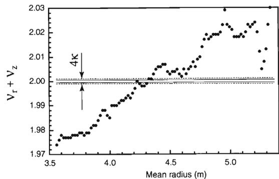
Fig. 2. Dots represent calculated  $\nu_r + \nu_z$  values for the SRC with an ion of 400 MeV/nucleon and  $A/q = 2$ . One dot corresponds to 4 or 5 turns. The area between the solid lines shows resonance band ( $2\kappa$ ). The area between the dashed lines is the area where the amplitude of oscillation may increase due to the resonance ( $4\kappa$ ).
