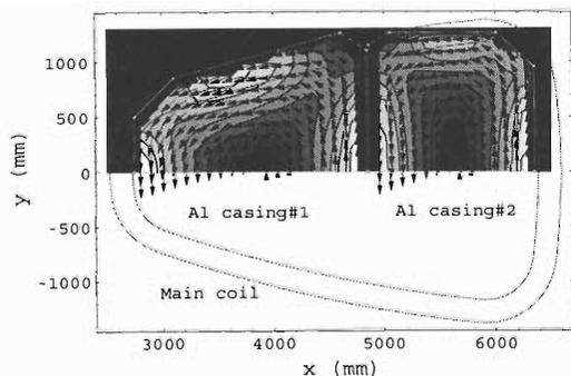
Fig. 3. Contour of  $|j|$  and vector plots of  $(j_x, j_y)$  for eddy current density in the Al casing of trim coils.
