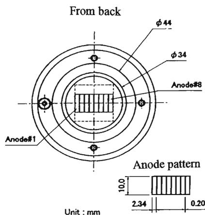
Fig. 2. A microchannel plate-mounted PMT with 8-separated anodes.
