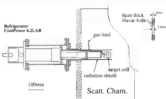
Fig. 1. View of liquid hydrogen target.
