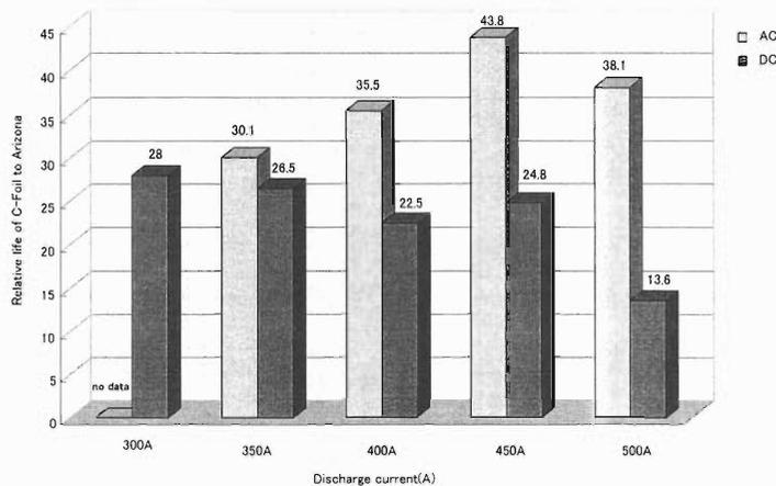
Fig. 3. Dependence of C-foil lifetime on the discharge current.
