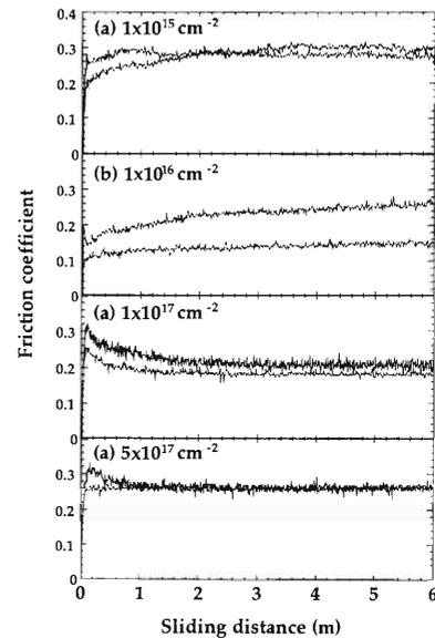
Fig. 1. The results of friction coefficient measurement in the pin-on-disk sliding test with an alumina counterface at a load of 5 N.
