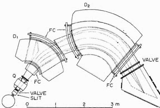
Fig. 1. Plane view of the high-resolution magnetic spectrograph PA.
