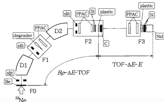
Fig. 1. Schematic depiction of the experimental setup.
