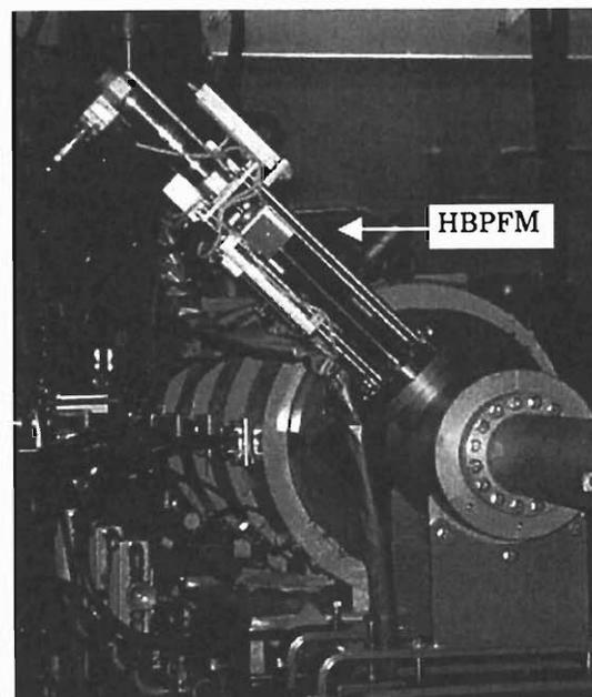
Fig. 2. The HBPFM located downstream of the QT7A1d. The fluorescence screen is monitored by a TV camera through the glass window located at the opposite side of the HBPFM.
