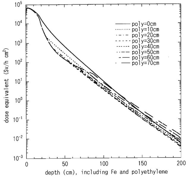
Fig. 3. Dose equivalent distribution in a 17-cm-thick-iron+polyethylene+ordinary-concrete slab. The irradiating neutrons are produced by 6.25-MeV/nucleon  $^{12}\text{C}$  beam bombardment on copper.
