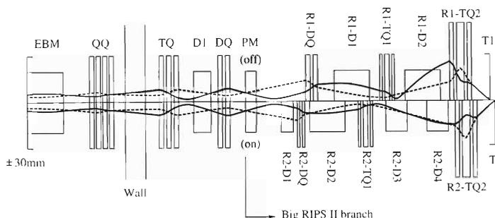
Fig. 3. First-order beam envelopes for the beam line from SRC to BigRIPS I and II. Solid (dashed) lines represent the horizontal (vertical) envelopes.
