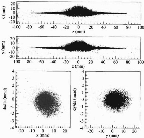
Fig. 2. Transverse phase-space distribution of the unstable bunched beam at 49 ms.
