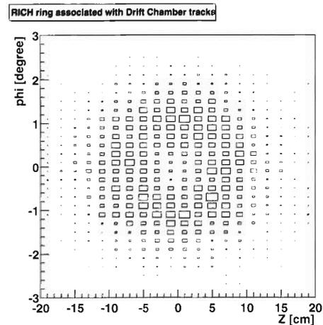
Fig. 1. Contour plot of RICH hits relative to the projected ring centroid from tracking, summed over many tracks.
