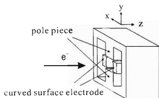
Fig. 1. Schema of spin rotator. The origin of the coordinates is the center of the spin rotator.
