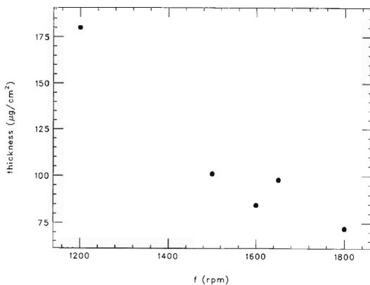
Fig. 4. Thickness of the liquid film as a function of rotating frequency of the disc.
