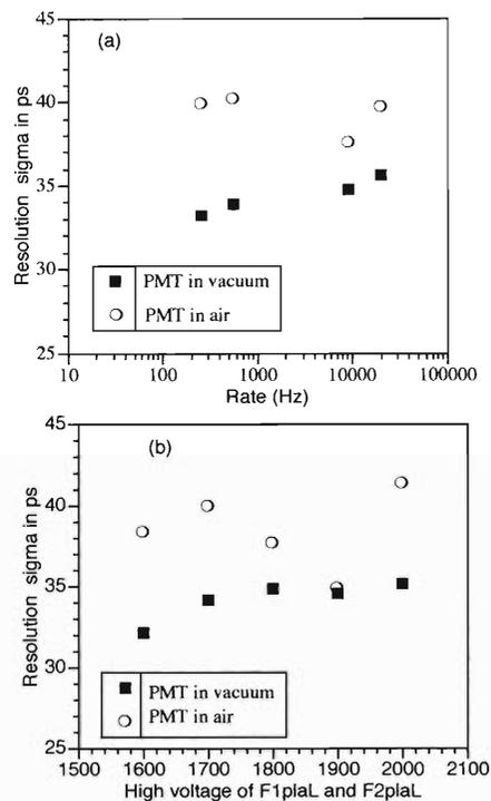
Fig. 1. Intrinsic time resolution comparison of PMT developed for use in vacuum and PMT used in air, (a) as a function of counting rate, and (b) as a function of PMT high voltage.
