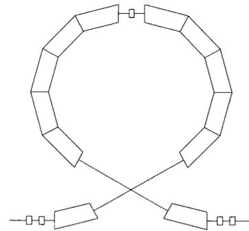
Fig. 5. The concept of an insertion device to lower the transition gamma.
