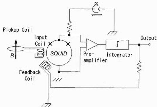
Fig. 3. Circuit diagram of a SQUID and flux-locked loop.
