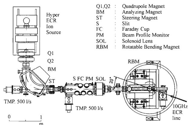
Fig. 1. Top view of the Hyper ECR ion source and the beam transport line to the rotatable bending magnet. The beam line was set to have a  $20^\circ$  deviation angle from that of the conventional ECR.
