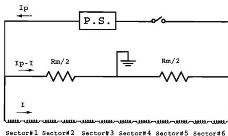
Fig. 1. Principal electric circuit for all superconducting main coils of all six sectors of SRC.
