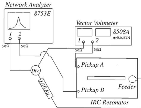
Fig. 1. Schematic view of an electric field measurement by a perturbation method.
