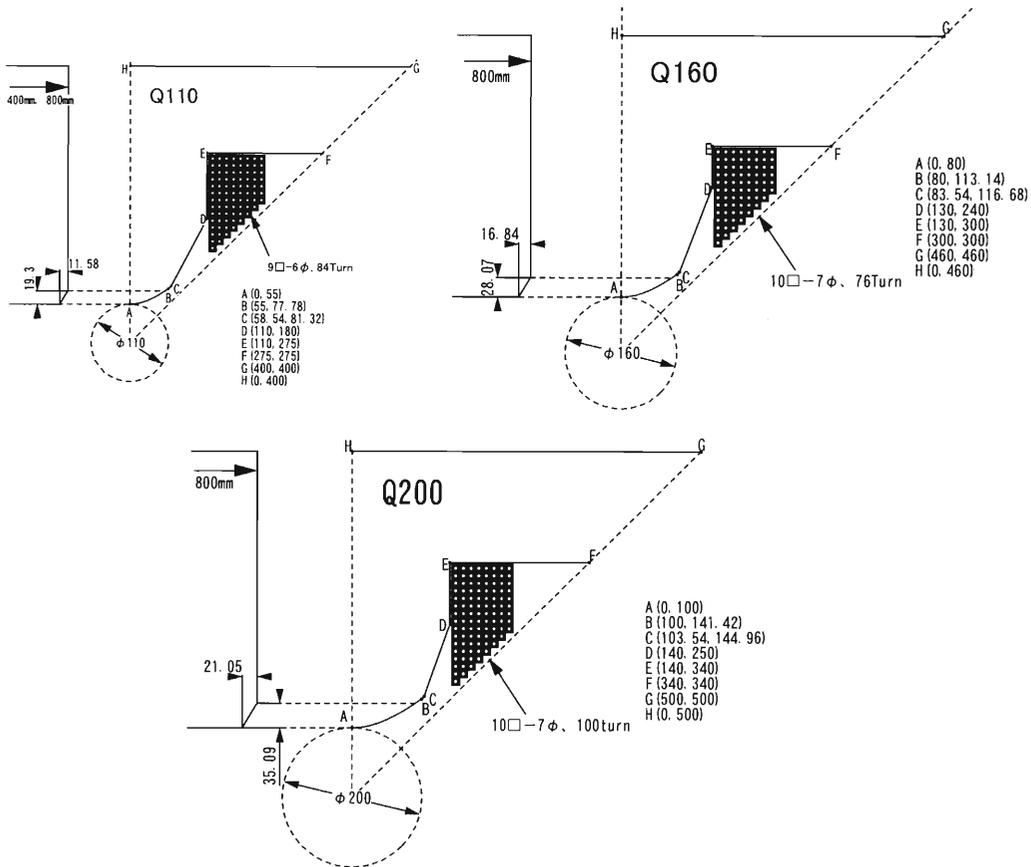
Fig. 1. Cross-sectional view of the quadrupole magnets, Q110, Q160 and Q200. Half of the poles and the coils are drawn. Letters correspond to the points on the Cartesian coordinates located at the origin in the center of the Bore radius. The shapes of pole end are also drawn.
