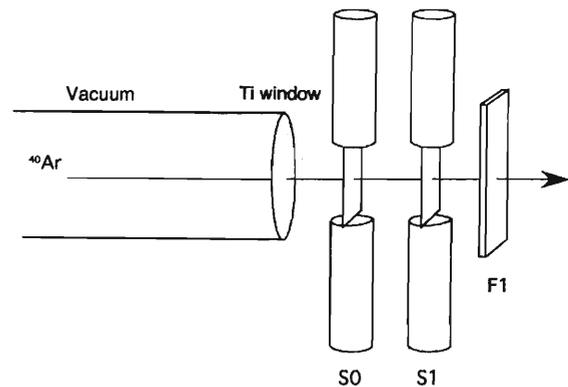
Fig. 1. Experimental setup for study of radiation hardness of scintillation detector.
