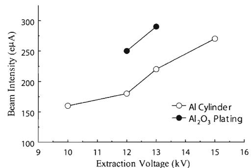
Fig. 2. Beam intensity of  $\text{Ar}^{11+}$  as a function of extraction voltage. Open and closed circles are the results by using Al cylinder method and  $\text{Al}_2\text{O}_3$  plating method, respectively.
