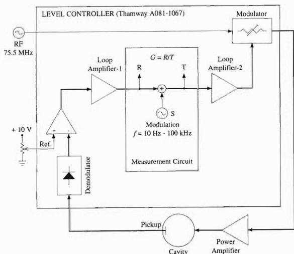
Fig. 1. Simplified block diagram of the feedback control system of cavity voltage of the CSM.
