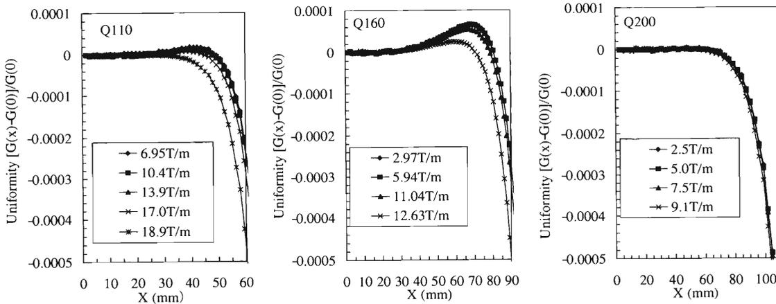
Fig. 3. Uniformity of the field gradient for Q110, Q160 and Q200. The horizontal axis indicates the distance from the center of the Bore radius.
