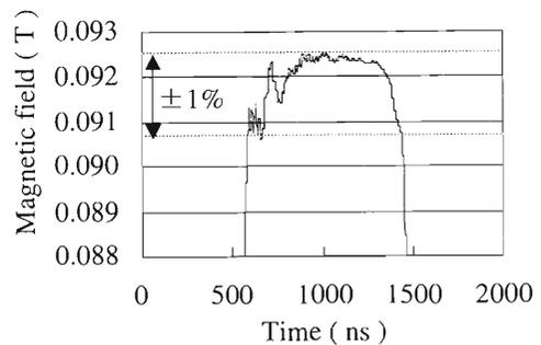
Fig. 2. Magnetic field at the flat-top.
