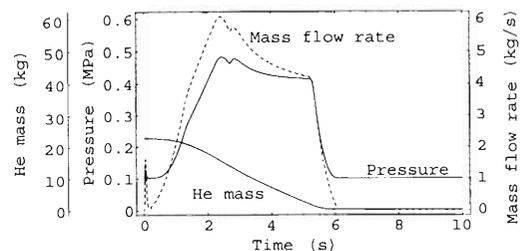
Fig. 4. Pressure rise and residual He mass in the coil vessel, and mass flow rate in pipe after a quench.
