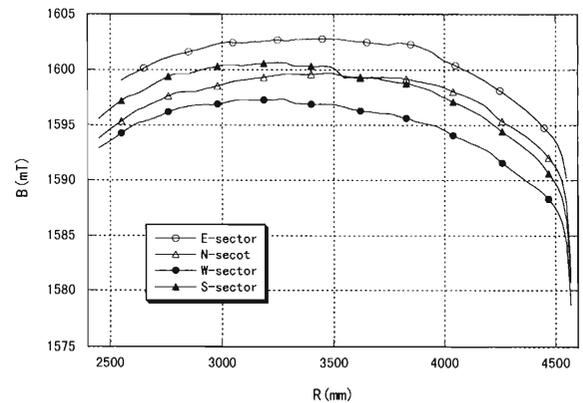
Fig. 2. Difference of the magnetic field distributions among four sector magnets at the main coil current of 290 A.
