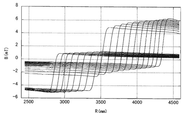
Fig. 3. Trim coil field distributions along the sector centerline at the base field of 1.6 T. The current values are  $-200$  A for the inner 8 coils and  $250$  A for the outer 12 coils, which are half of the nominal currents. The minus sign of the current indicates that the current direction is the reverse of that of the main coil.
