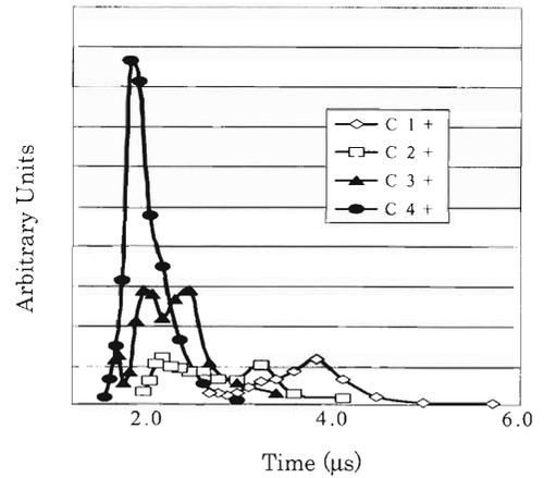
Fig. 4. Pulse time structure for each charge state of the carbon ions.
