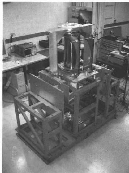
Fig. 4. The X-Z stage which is moved by four stepping motors in the X-Y plane. The X-Y stage is remotely controlled by a personal computer (PC). The X-Y stage is equipped with a Helmholtz coil, which can produce a uniform magnetic field of 1 mT.
