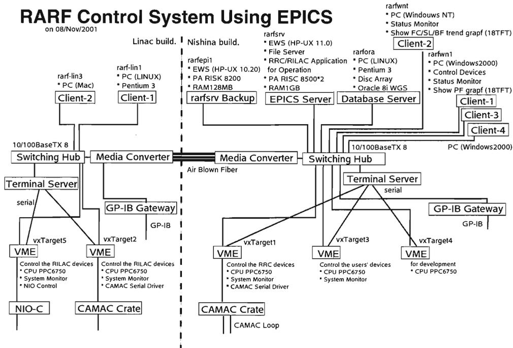
Fig. 2. Client PC configuration for EPICS at the RRC control room.
