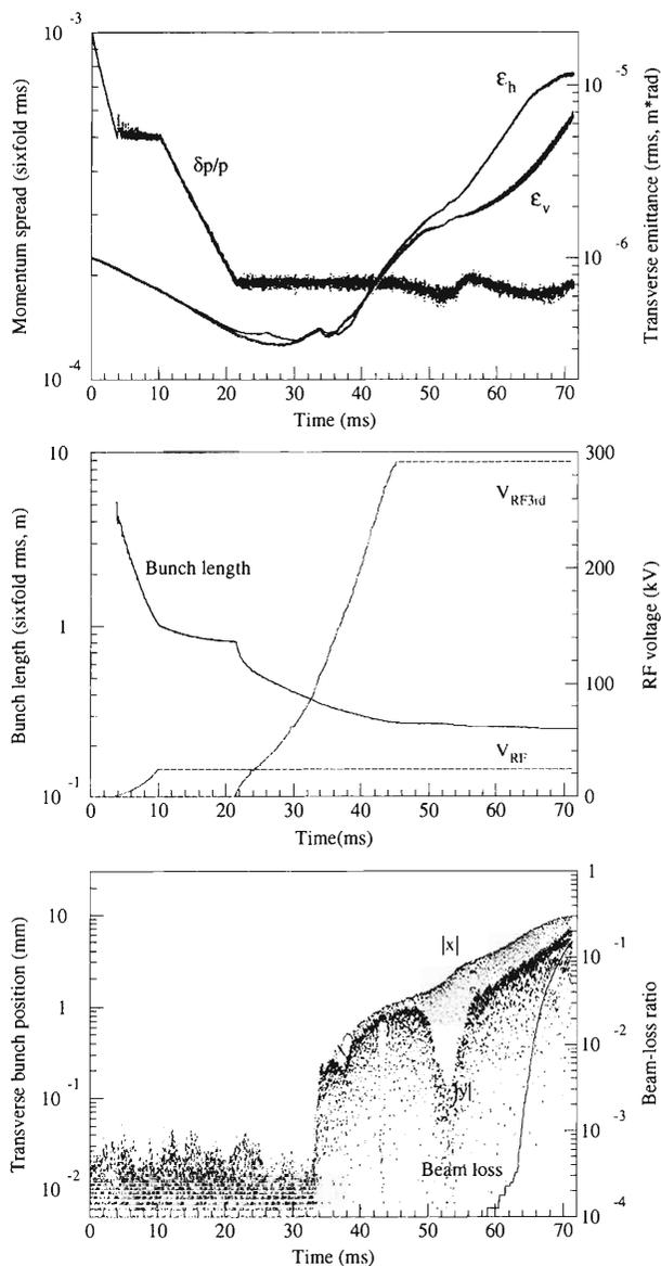
Fig. 1. Time evolution of the EC bunching of a  $^{238}\text{U}^{92+}$  ion beam of 4 mA at 150 MeV/u.
