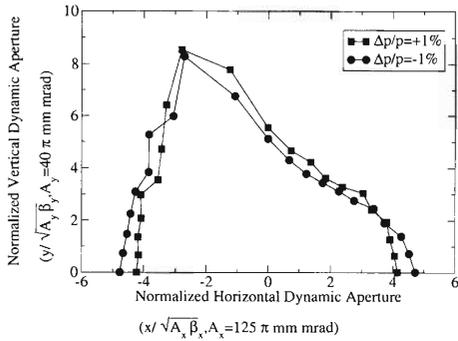
Fig. 3. Dynamic aperture of the ACR at the center of the electron cooling (EC) section with  $\Delta p/p = \pm 1\%$ . The particles were tracked by MAD8<sup>3)</sup> for various initial transverse positions  $(x, y)$  normalized by the beam size.
