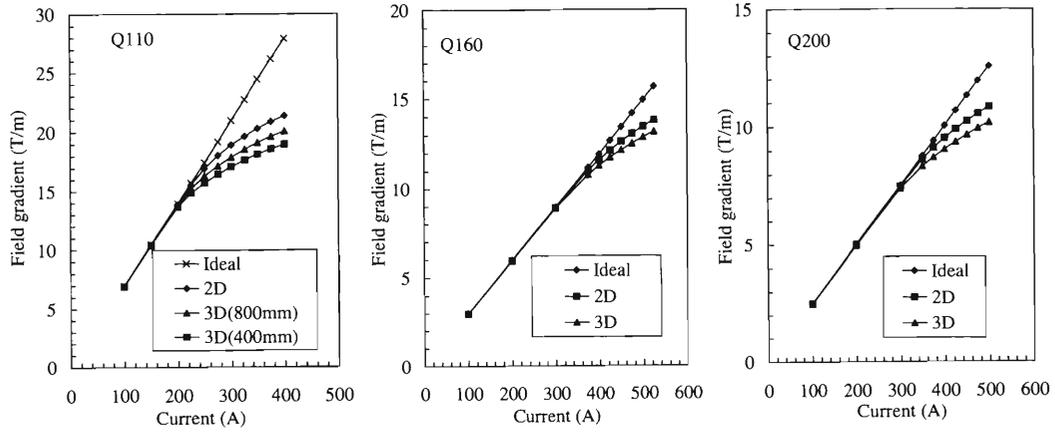
Fig. 2. Excitation curve of the field gradient for Q110, Q160 and Q200. Q110 has two pole lengths, 400 mm and 800 mm.
