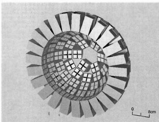
Fig. 2. Schematic of the CsI(Tl) array which consists of 312 crystals.
