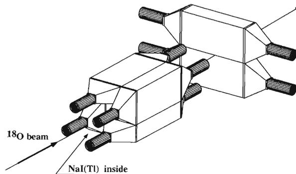
Fig. 2. Schematic view of the reaction suppressor. The total E detector is placed inside the suppressor.
