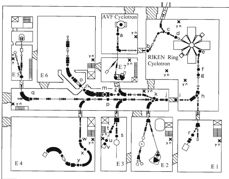
Fig. 1. Layout of the RIKEN Ring Cyclotron Facility as of 2001. Measured locations of residual radioactivities along the beam lines are shown by bullets **a–y**.
