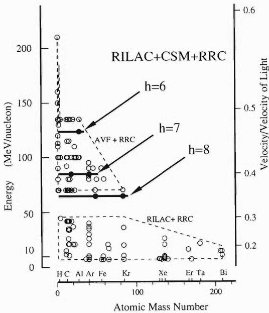
Fig. 1. Performance of RRC. The two regions surrounded by dashed lines are the conventional acceptances for the AVF+RRC and RILAC+RRC. The open circles denotes the beams accelerated previously. The three solid lines shows the beams obtained with the new scheme of RILAC+CSM+RRC and the solid circles are beams shown in Table 1.
