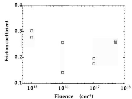
Fig. 2. The friction coefficient of the specimens implanted with W at a sliding distance of 6 m.
