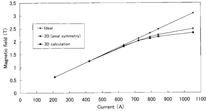
Fig. 3. Excitation curves of the magnetic field by the 3D calculation. The ideal excitation curve and the results of 2D calculation are also plotted.
