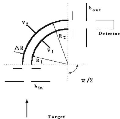
Fig. 2. Structure of the electric analyzer.
