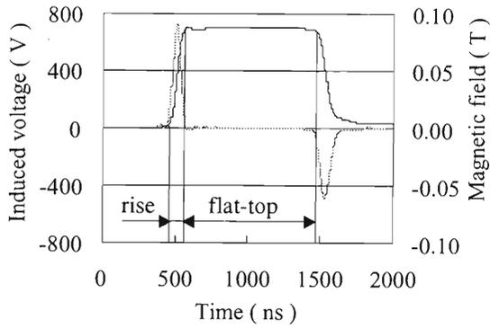
Fig. 3. Magnetic field and induced voltage with the capacitors.
