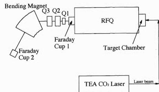
Fig. 2. Layout of the experimental setup.
