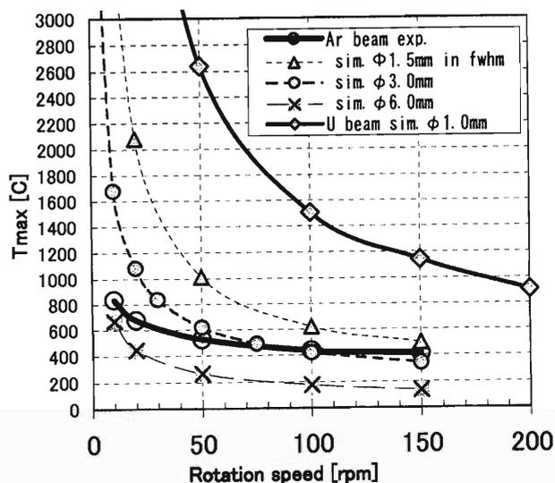
Fig. 1. Maximum temperature of the beam spot at various rotation speeds of the carbon target disk. Experimental data (thick straight line) and simulation results for various beam spot sizes (dotted lines) are shown for the  $^{40}\text{Ar}$  beam test experiment. The estimation for  $^{238}\text{U}$  beam (thick dotted line) is also indicated.
