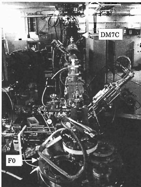
Fig. 1. The E7 beam line. The K70-AVF cyclotron beam is transmitted from the upper floor and is bent by DM7C in the E7. The quartet-Q magnets and CRIB-F0 target are seen in front sight. Vacuum isolation between the E7 beam line and the K70-AVF cyclotron can be realized with a rotary shutter RC-CE7 with the gate valve function.
