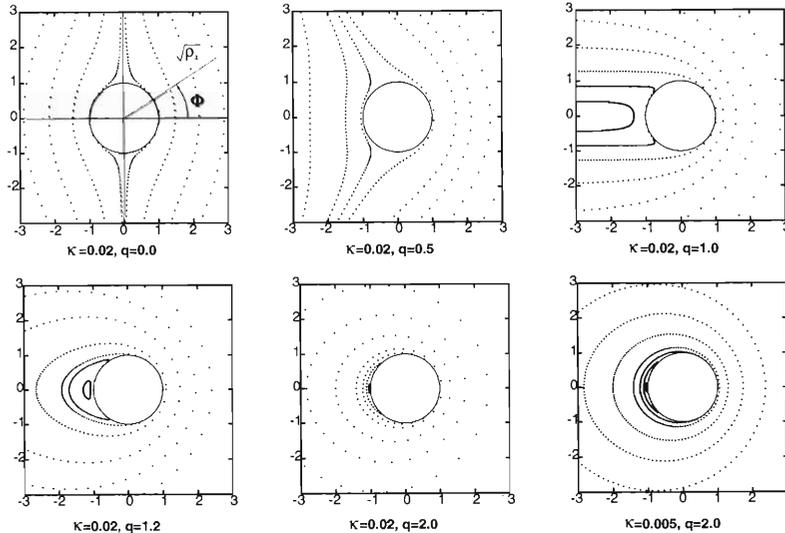
Fig. 1. Phase-space plots for the  $\nu_r + \nu_z = 2$  resonance with polar coordinates  $\sqrt{\rho_x}$  and  $\Phi$ . Consecutive points are plotted at intervals of  $\Delta\theta = 2\pi$ . If  $|q| > 1$ , the equations of motion have oscillating solutions.
