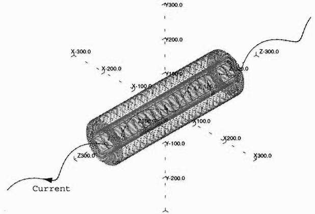
Fig. 3. Schematic drawing in the case of a single helical coil placed inside a cylindrical hole in iron.
