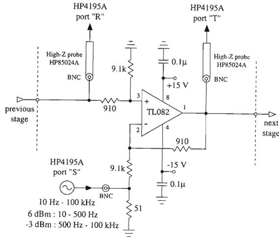
Fig. 3. Schematic drawing of the measurement circuit.
