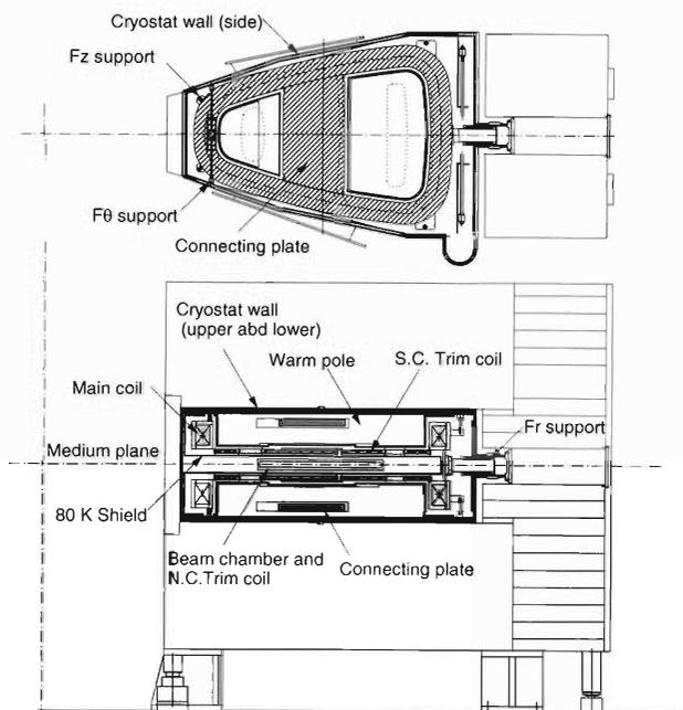
Fig. 1. Cross-sectional and plan views of the SRC sector magnet.
