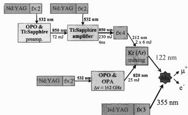
Fig. 2. Schematic diagram of the laser system which has been developed for the resonant ionization of muonium atom.
