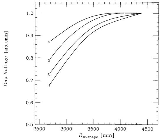
Fig. 3. Voltage distributions as a function of averaged radius of the beam orbit for (1) 18 MHz, (2) 28 MHz, (3) 36 MHz, and (4) 41 MHz. The gap voltage is maximum at the extraction radius.
