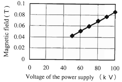
Fig. 5. Dependence of the magnetic field strength on the voltage of the power supply.
