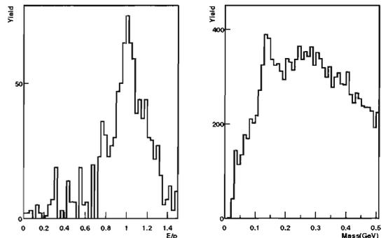
Fig. 2. (Left) Ratio of measured energy and momentum for electron sample at PHENIX Au+Au Collision  $\sqrt{s_{NN}} = 130 \text{ GeV}$ . (Right) Two-photon invariant mass spectrum at PHENIX Au+Au Collision  $\sqrt{s_{NN}} = 130 \text{ GeV}$ .
