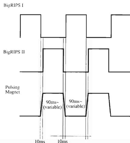
Fig. 1. Operation pattern of the pulsing mode.
