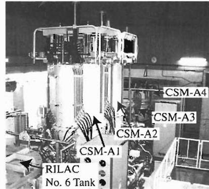
Fig. 1. Photograph of the CSM A1–A4 cavities.
