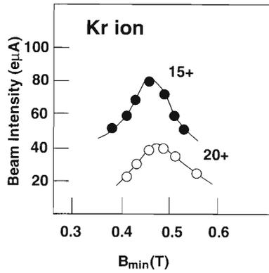
Fig. 4. Beam intensities of Kr ions as a function of  $B_{\min}$ .
