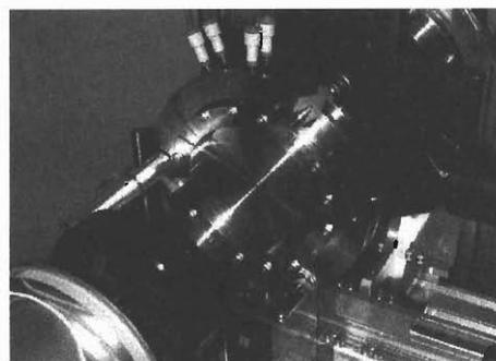
Fig. 2. Wedge shaped energy degrader of variable angle and thickness.
