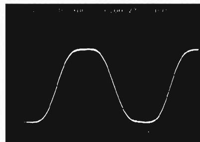
Fig. 6. Typical waveform of the flat-top voltage measured by the dee-voltage pickup. The fundamental frequency was 16.3 MHz and the 3rd-harmonic frequency was 48.9 MHz. The fundamental voltage was 50 kV.
