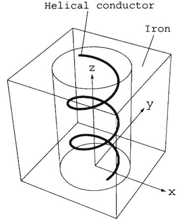
Fig. 1. Schematic view of a single helical coil placed inside a cylindrical hole in iron.
