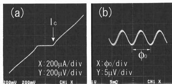
Fig. 2. Characteristics of SQUID; (a) current ( $x$ -axis) vs. voltage ( $y$ -axis) appears across the Josephson junctions of HTS SQUID, (b) relationship of the magnetic field  $B$  ( $x$ -axis) at the input coil with voltage ( $y$ -axis).
