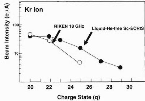
Fig. 2. Beam intensities of highly charged Kr ions. Closed and open circles are the beam intensities produced from SC-ECRIS and RIKEN 18 GHz ECRIS, respectively.
