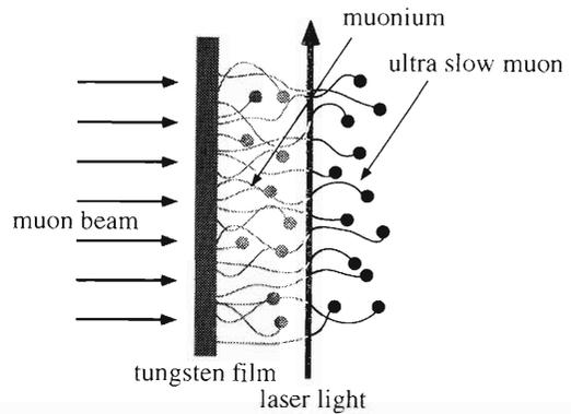
Fig. 1. Schematic diagram of the laser ionization method for generating slow muons.
