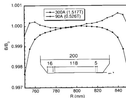
Fig. 2. Cross-sectional view of the dipole magnet and the radial distributions of magnetic fields are shown.
