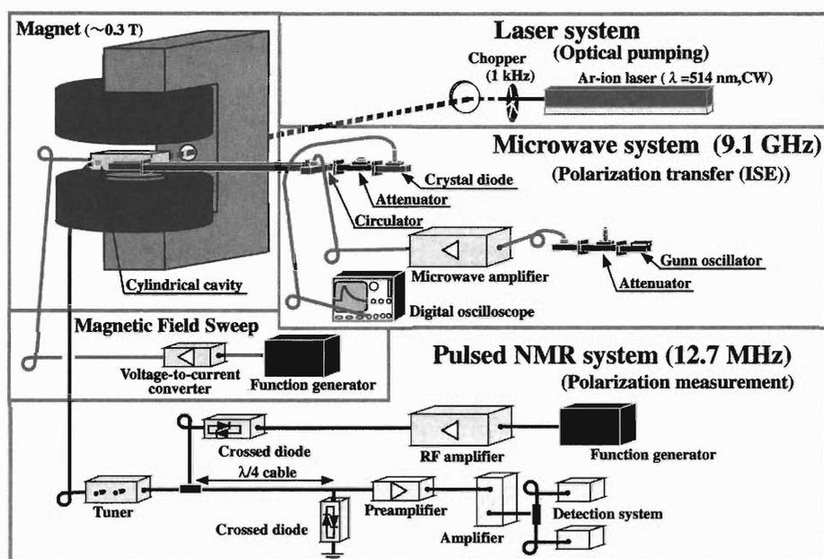
Fig. 1. Schematic of the proton polarizing system. The system consists of a magnet, a laser system for optical pumping, a microwave system and a magnetic field sweep system for polarization transfer, and a pulsed NMR system for polarization measurement.
