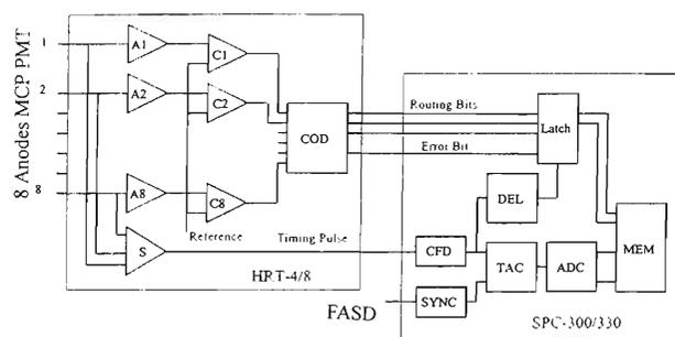
Fig. 1. System for time-correlated 8-channel photon counting for each ion striking. FASD: a fast secondary electron detector.<sup>1)</sup>
