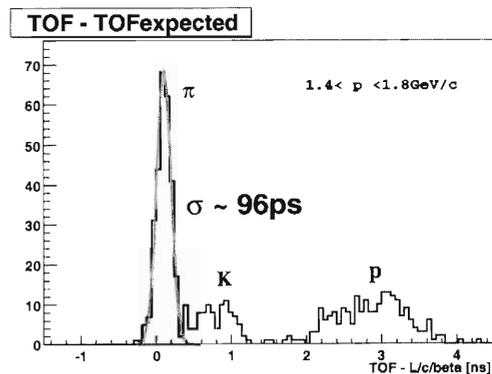
Fig. 2. The time-of-flight distribution in the momentum is  $1.4 < p < 1.8$  GeV/c for positively charged pions. The overall time-of-flight resolution of less than 100 ps is achieved.
