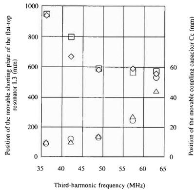
Fig. 3. Positions of the movable shorting plate and the coupling capacitor of the flat-top resonator as a function of the 3rd-harmonics frequency. Squares and circles represent the positions of the shorting plate and the coupling capacitor of the No. 1 resonator, respectively. Diamonds and triangles represent the positions of the shorting plate and the coupling capacitor of the No. 2 resonator, respectively.
