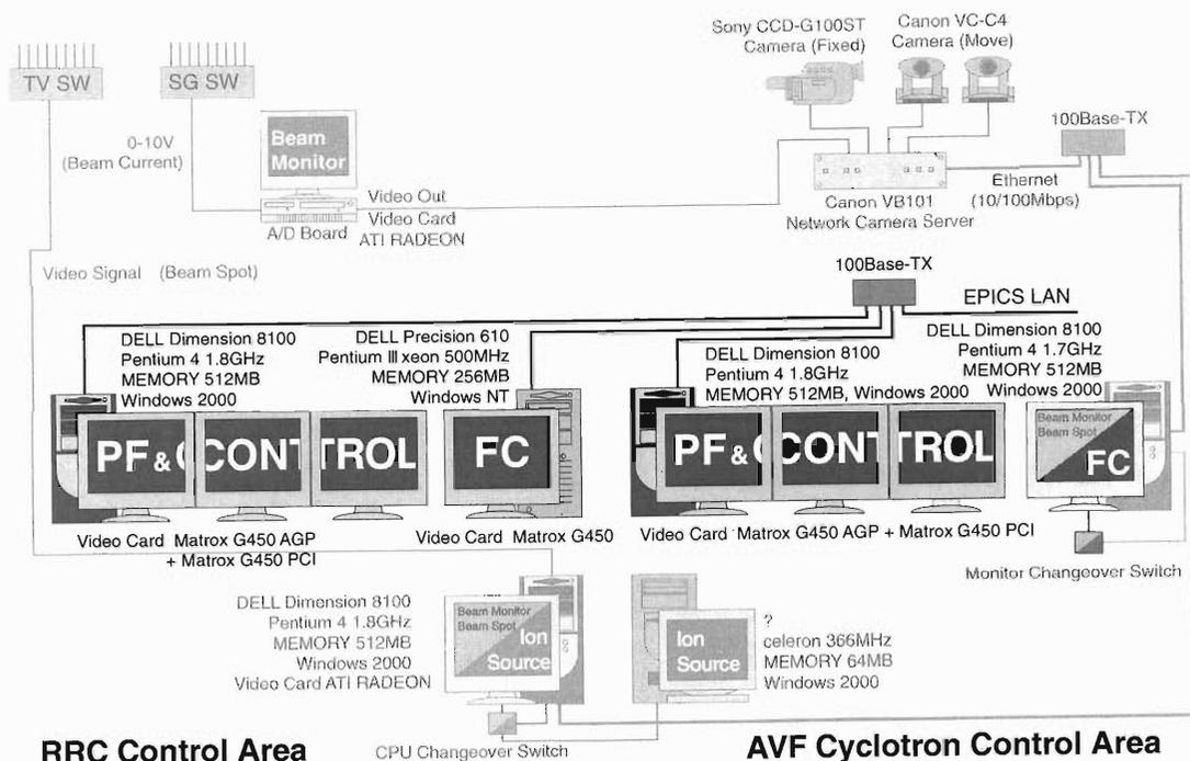
Fig. 1. Structure of the RARF control system using EPICS.
