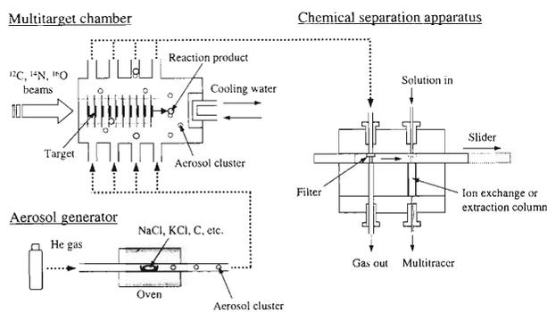
Fig. 1. Schematic of the gas-jet coupled multitarget system and the automated rapid chemistry apparatus.
