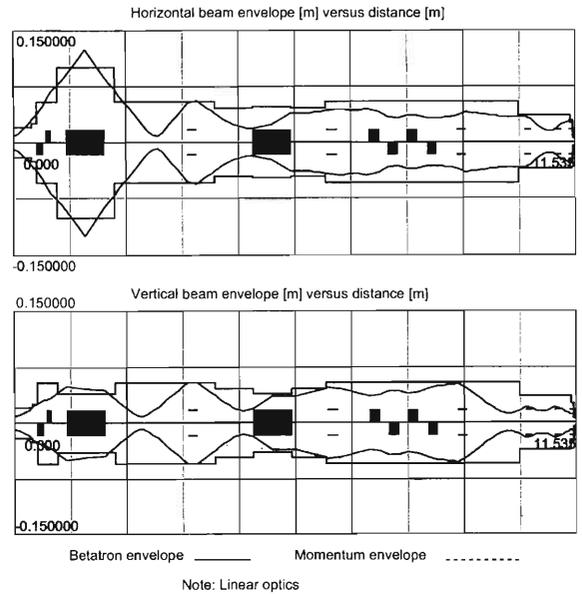
Fig. 2. First-order beam envelope along the injection line calculated for the  $^{14}\text{N}^{5+}$  beam:  $B\rho = 30 \text{ kGcm}$ .
