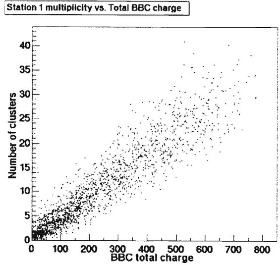
Fig. 3. Coincidence between multiplicity of clusters in muon tracker station 1 and total charge detected in the beam-beam counter measured in the Au-Au collisions at  $\sqrt{s_{NN}} = 200\ \text{GeV}$ .
