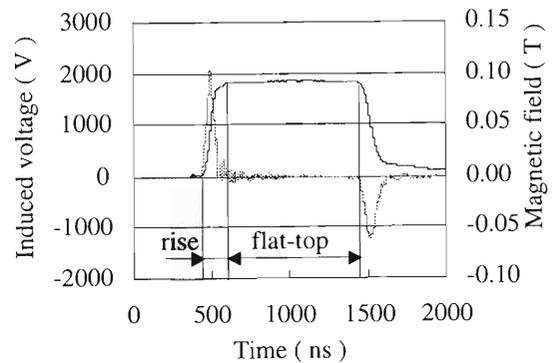
Fig. 1. Magnetic field and induced voltage.
