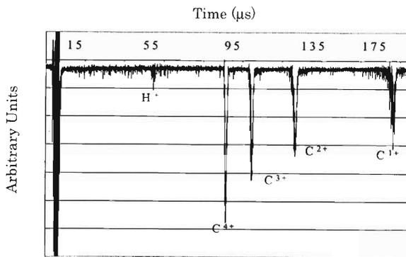
Fig. 3. Typical Ceratron signal.
