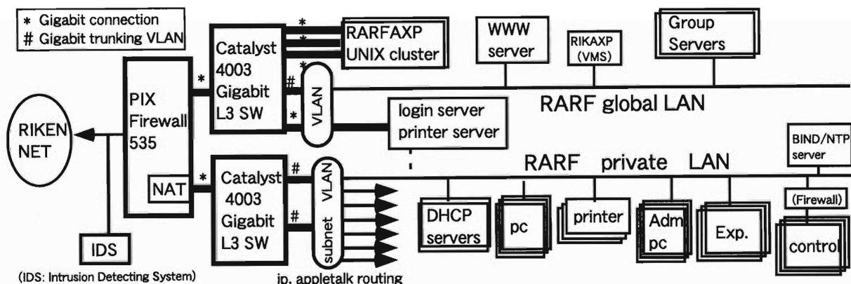
Fig. 1. Configuration of the RARF Advanced LAN.
