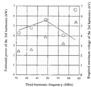
Fig. 5. Estimated power and the required maximum voltage of the 3rd harmonics. Circles represent the estimated power of the No. 1 resonator and triangles represent that of the No. 2 resonator. Solid line represents 1/9 of the required maximum fundamental acceleration voltage.
