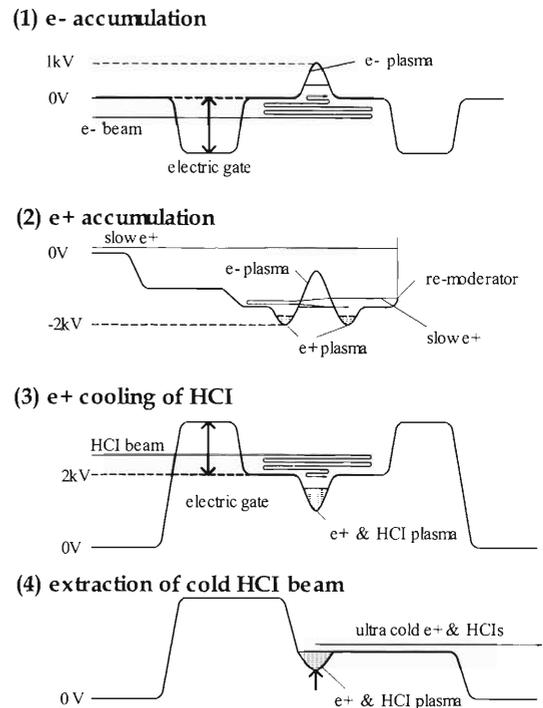
Fig. 1. Procedure of HCl cooling.
