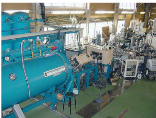
Fig.1 The Pelletron tandem accelerator and beamlines
