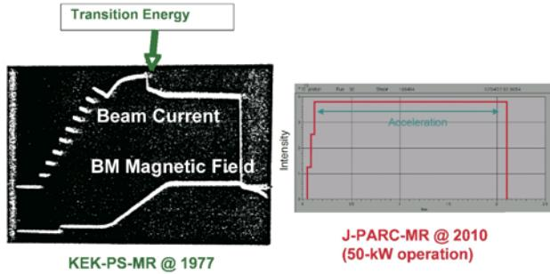
Figure 13: Beam current variation patterns during the injection and the energy ramping. The left is that of the KEK-PS MR (courtesy of KEK Archives Office), while the right is that of J-PARC MR. The original data points of the right figure were too thin to see. So, the data points were traced in a thick curve.
