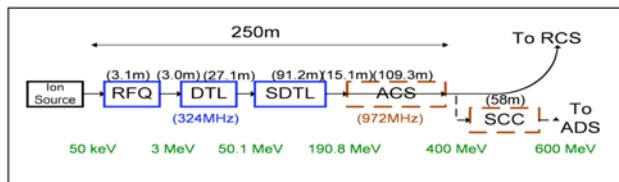
Figure 6: Scheme of J-PARC linac.
