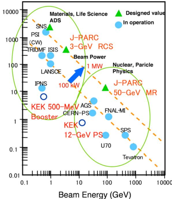
Figure 9: Beam currents and beam energies of the major proton accelerators in the world.
