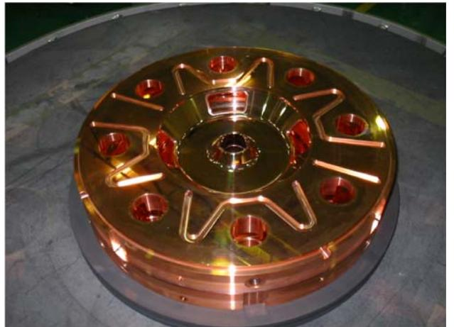
Figure 11: A half cell of the J-PARC ACS. The view is from the accelerating cavity side.
