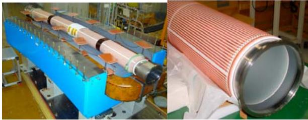
Figure 15: Ceramic chambers used for the J-PARC RCS. The left is for the bending magnet, while the right for the quadrupole magnets.
