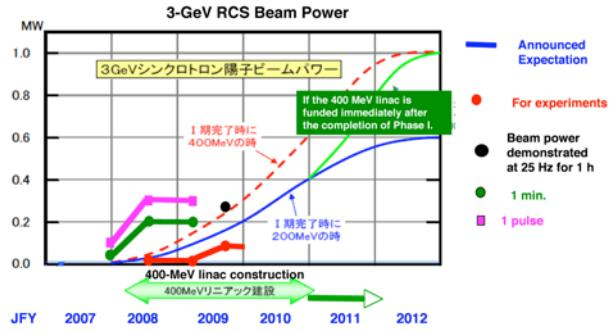
Figure 16: An expectation of the beam-power improvement as compared with the realized.
