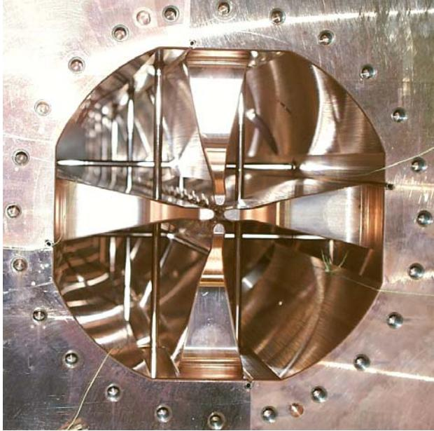
Figure 10: Inside view of the J-PARC linac. Bar-like objects are PISLs.
