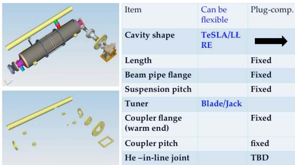
Figure 5: Sketch of the assembled ILC RF cavity. The lower part of the figure highlights the parts of the assembly that must interface with other cavities or other components.
