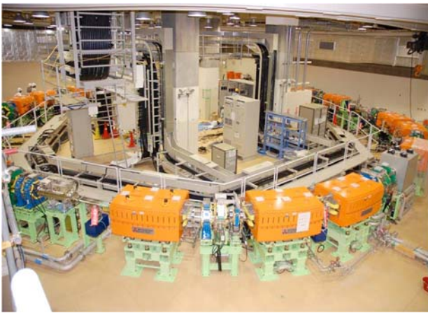
Figure 13: Synchrotron ring with a circumference of 63 m.
